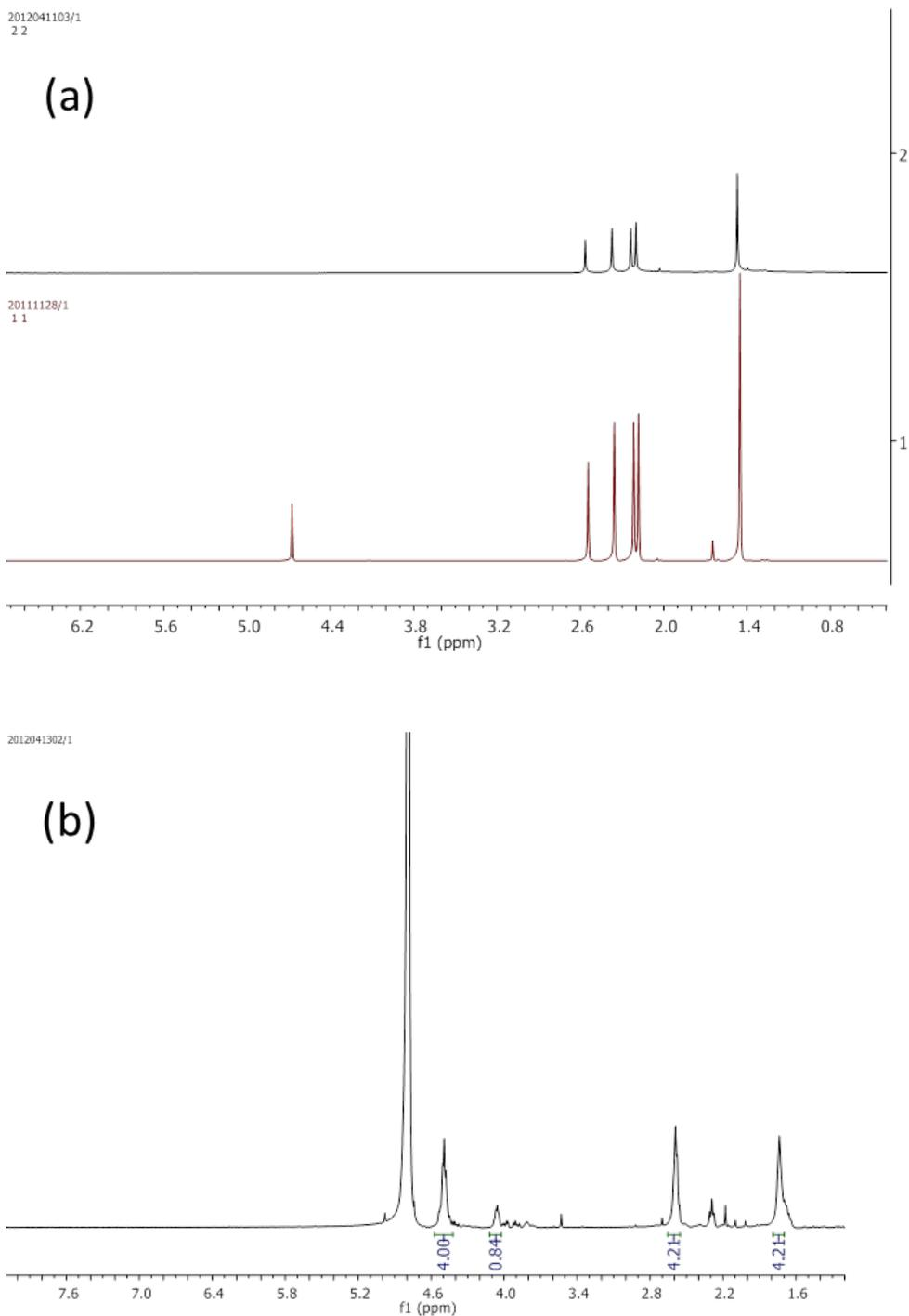
**Figure 6.** NMR spectra of the reduction products after polymer reduction by sodium dithionite. (a) NMR spectra of the organic solvent-soluble components after polymer reduction (top), and synthesized benzoquinone lactone (bottom) in  $\text{CDCl}_3$ . (b) NMR spectrum of the water-soluble components after polymer reduction in  $\text{D}_2\text{O}$ .
