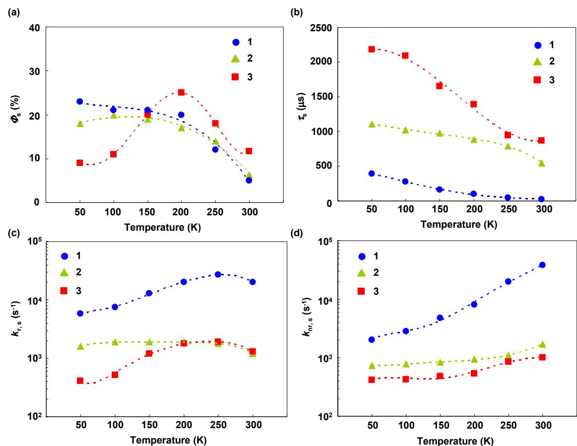
Fig. S4 (a) Temperature dependence of  $\Phi_s$  for **1** (blue), **2** (green) and **3** (red) in PYD2 films. (b) Temperature dependence of the lifetime ( $\tau_s$ ) of **1** (blue), **2** (green) and **3** (red) in PYD2 films. (c) Temperature dependence of the rate of radiative decay ( $k_{r,s}$ ) for **1** (blue), **2** (green) and **3** (red) in PYD2 films. (d) Temperature dependence of  $k_{nr,s}$  for **1** (blue), **2** (green) and **3** (red) in PYD2 films.
