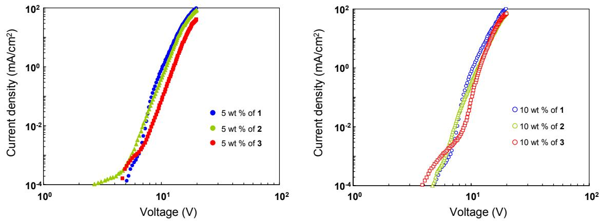
Fig. S6 *J-V* characteristics for OLEDs with the structure ITO/PEDOT:PSS (40 nm)/X wt% of Cu complex:PYD2 (30 nm)/DPEPO (50 nm)/LiF (0.7 nm)/Al (100 nm).
