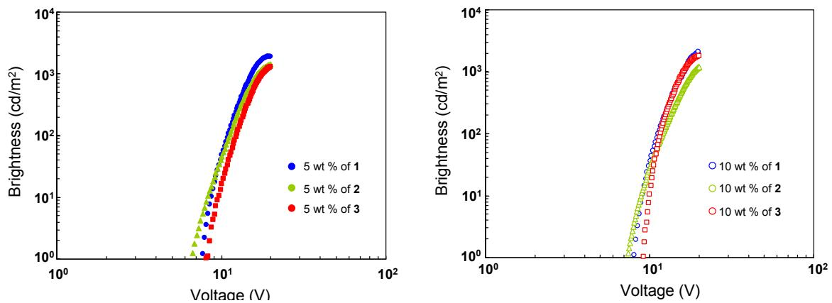
Fig. S7 *L-V* characteristics for OLEDs with the structure ITO/PEDOT:PSS (40 nm)/X wt% of Cu complex:PYD2 (30 nm)/DPEPO (50 nm)/LiF (0.7 nm)/Al (100 nm).
