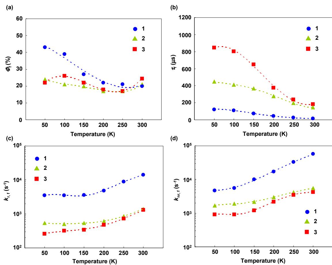
Fig. S3 (a) Temperature dependence of  $\Phi_f$  for **1** (blue), **2** (green) and **3** (red) in PYD2 films. (b) Temperature dependence of the lifetime ( $\tau_f$ ) of **1** (blue), **2** (green) and **3** (red) in PYD2 films. (c) Temperature dependence of the rate of radiative decay ( $k_{r,f}$ ) for **1** (blue), **2** (green) and **3** (red) in PYD2 films. (d) Temperature dependence of  $k_{nr,f}$  for **1** (blue), **2** (green) and **3** (red) in PYD2 films.
