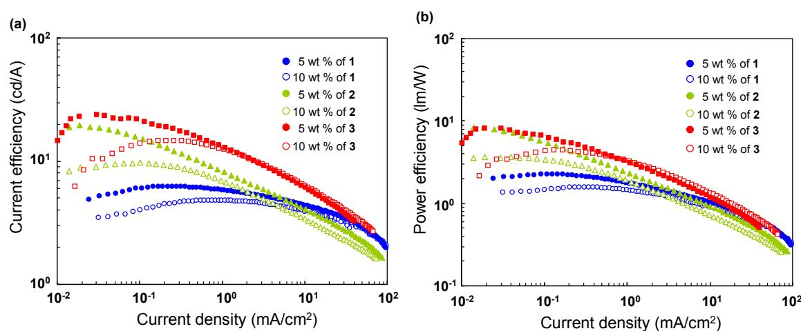
Fig. S5 (a) Dependence of current efficiency on current density for OLEDs with the structure ITO/PEDOT:PSS (40 nm)/X wt% of Cu complex:PYD2 (30 nm)/DPEPO (50 nm)/LiF (0.7 nm)/Al (100 nm). (b) Dependence of power efficiency on current density for OLEDs with the structure ITO/PEDOT:PSS (40 nm)/X wt% of Cu complex:PYD2 (30 nm)/DPEPO (50 nm)/LiF (0.7 nm)/Al (100 nm).
