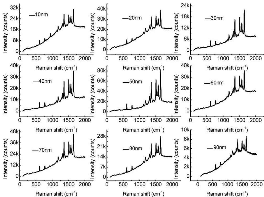
**Fig. S4** Raman spectra of paper with silver thickness from 10nm to 90nm.
