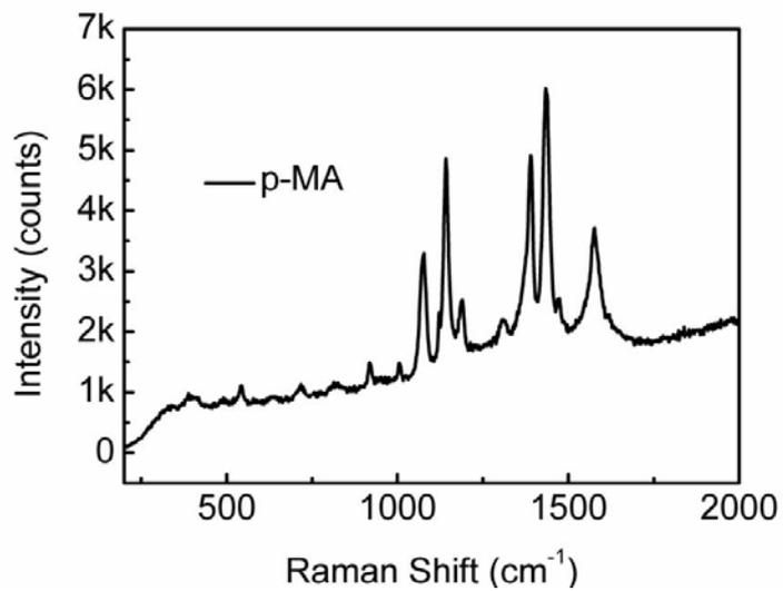
Fig. S1 SERS spectrum of p-Mercaptoaniline (p-MA) with a concentration of  $10^{-6}$  M on the Ag/paper substrate.
