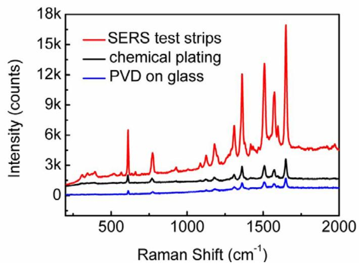
**Fig. S8** Comparison of the SERS spectra of R6G of  $10^{-6}$ M on the test strips, chemical silverplating on glass and the PVD Ag film on glass.
