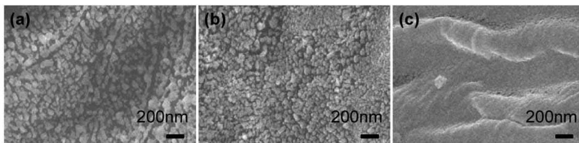
**Fig. S3** SEM images of the paper covered with silver of (a) 5nm; (b) 10nm; (c) 20nm.
