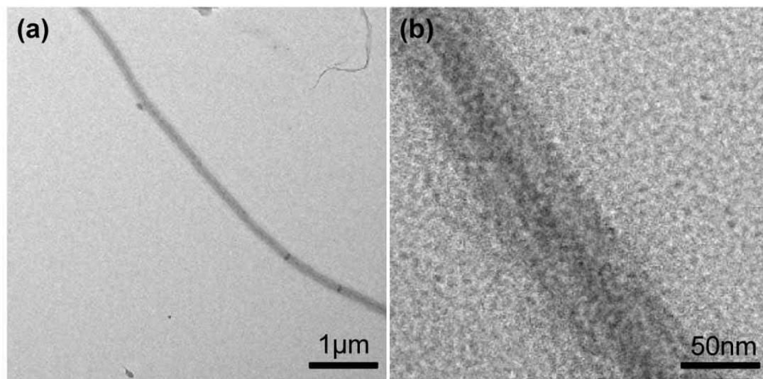
**Fig. S6** TEM image of the nanofibrils separated from the printing paper (a) and the magnified image (b).
