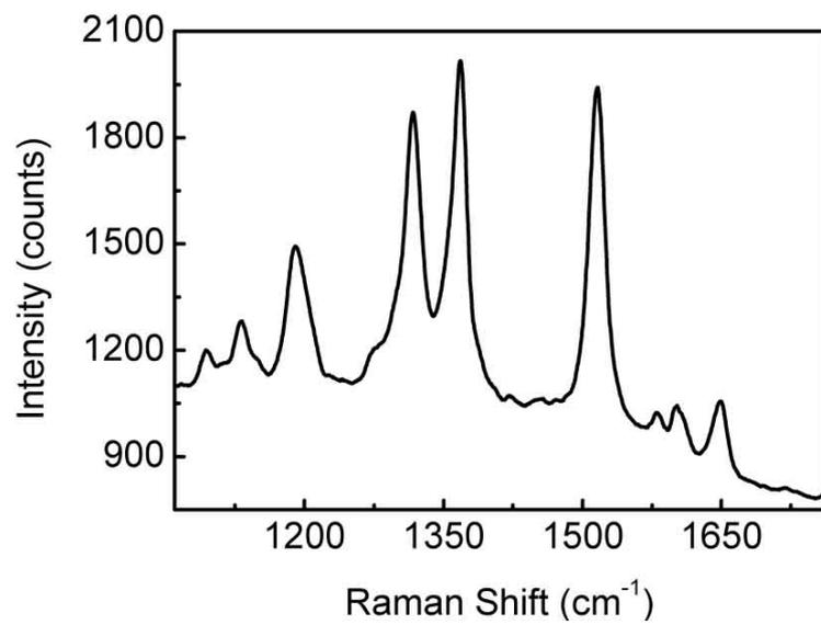
Fig. S2 SERS spectrum of the R6G of  $10^{-6}$ M on Ag/paper, the excitation wavelength is 785 nm.
