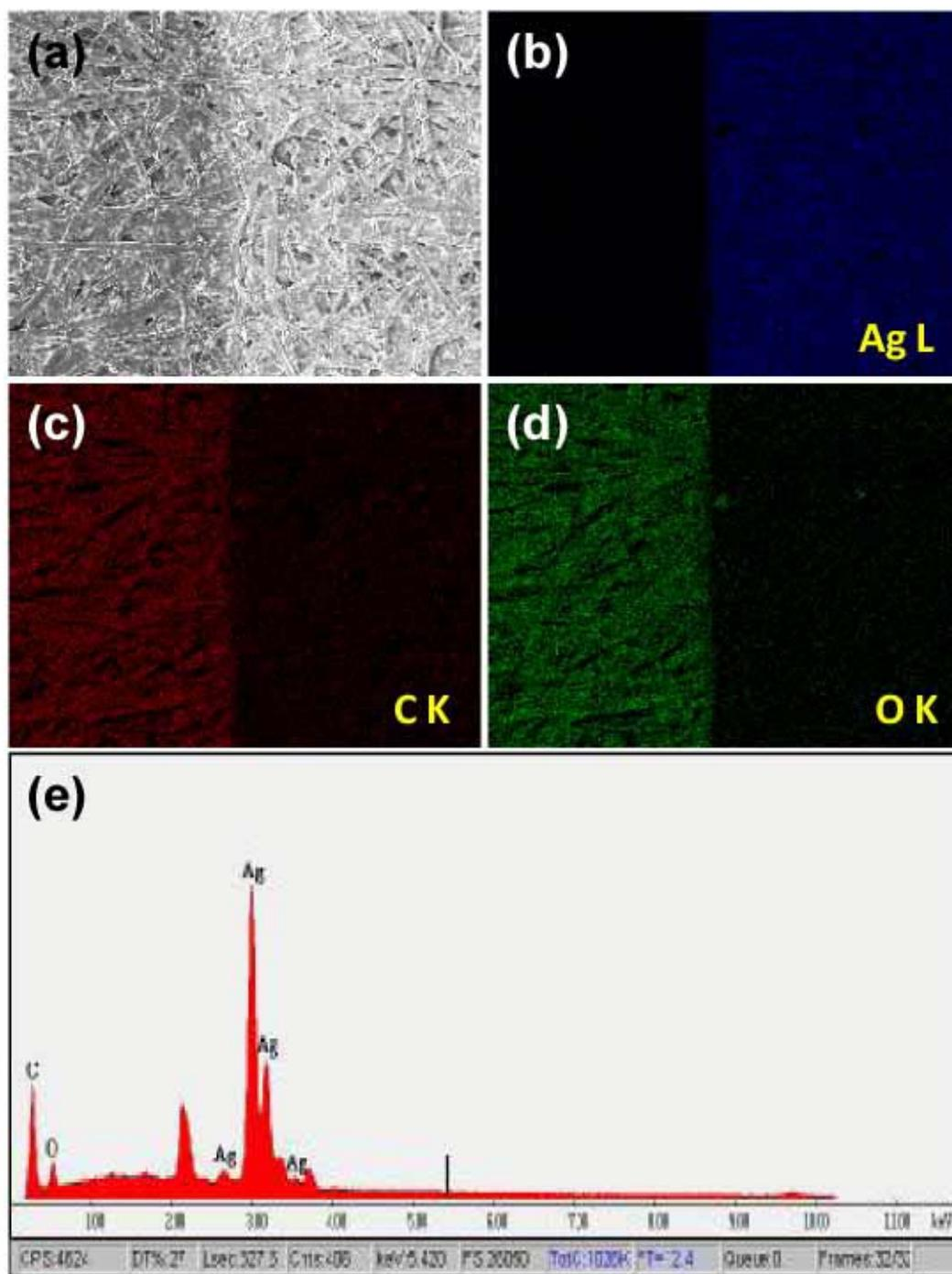
**Fig. S11** (a) SEM image of the boundary of the paper with and without silver coating; the EDX of the (b) Ag maps (c) C maps (d) O maps corresponding to the SEM image; (e) EDX spectrum of the silver coated paper.
