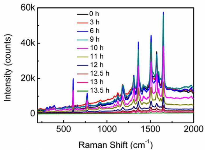
**Fig. S9** Time dependent SERS intensity of the new-made test strips.
