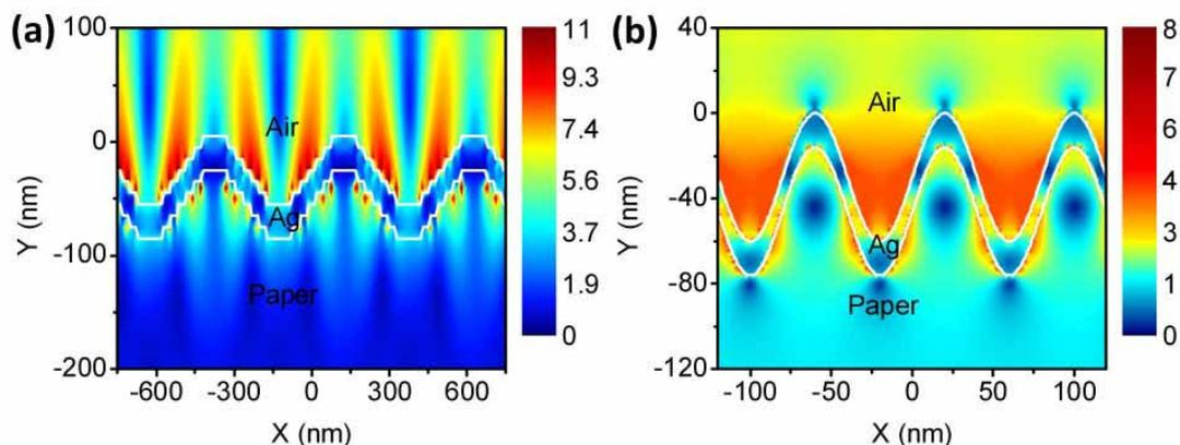
**Fig. S7** Electric field component  $E_x$  distribution simulations of (a) silver coated wrinkles with intervals of 500nm; (b) silver coated nanofibrils of 80nm width. The incident laser wavelength is 514 nm.
