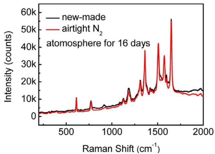
**Fig. S10** The SERS spectra of the new-made test strips and that placed in airtight N<sub>2</sub> atmosphere for 16 days.
