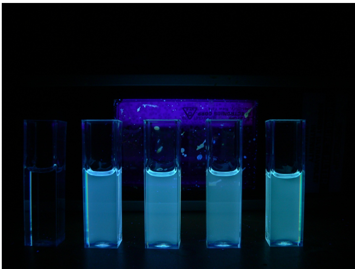
Fig. S6 Several samples of GQDs in toluene under UV illumination. The leftmost one is toluene for comparison.
