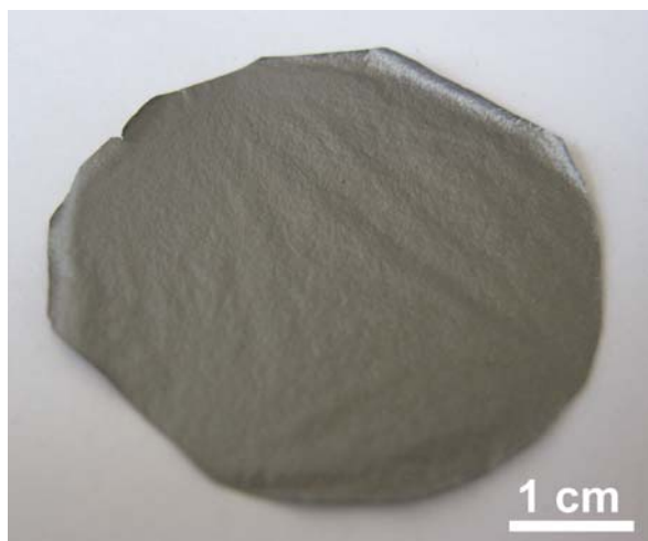
Fig. S2 Digital photo of a compact graphene film (CGF) fabricated by a routine filtration method.
