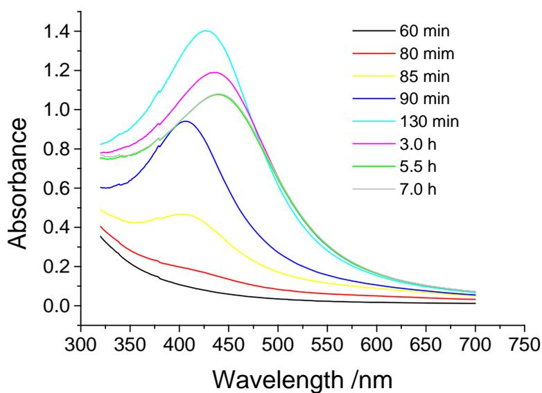
**Figure S2.** UV-vis monitoring of the FSDNA-templated AgNPs during an aging process at 37 °C. Note that the absorbance curve became constant after a 5.5 h reaction and aging (1 h NaBH<sub>4</sub>-based reduction in ice-water bath and 4.5 h aging at 37 °C).
