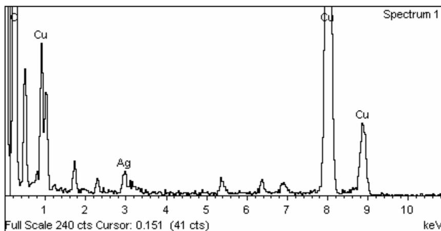
**Figure S1.** Energy dispersive X-ray spectroscopic (EDX) analysis of the silver nanoparticles supported on carbon coated copper grid, which evidenced the existence of silver element.
