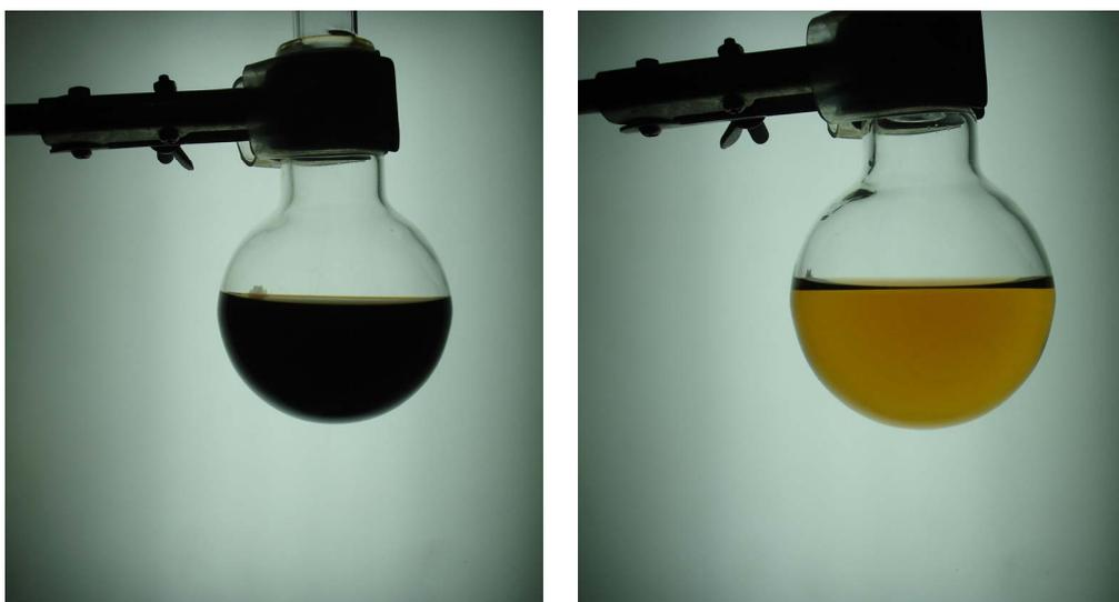
**Figure S6.** As-synthesized FSDNA stabilized silver nanoparticles (left picture) and its ten-time dilution (right picture).
