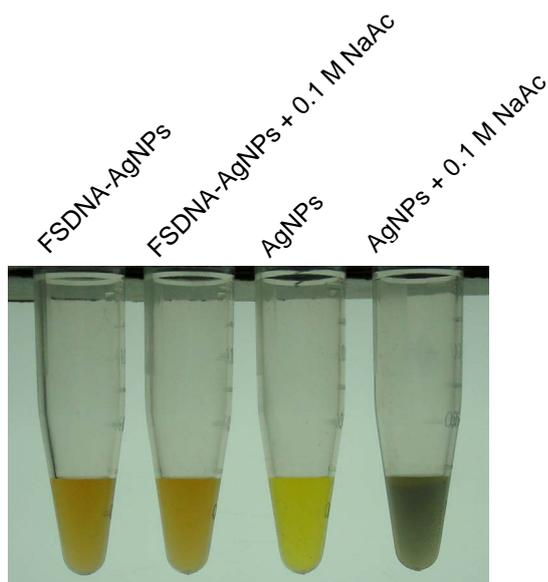
**Figure S5.** Salt-resistance test of the AgNPs synthesized in the presence or absence of FSDNA.
