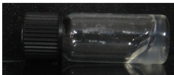
Fig. S-5. An optical image of a weak gel containing 0.5 wt% of 4 itself in PBS solution (pH = 7.4)
