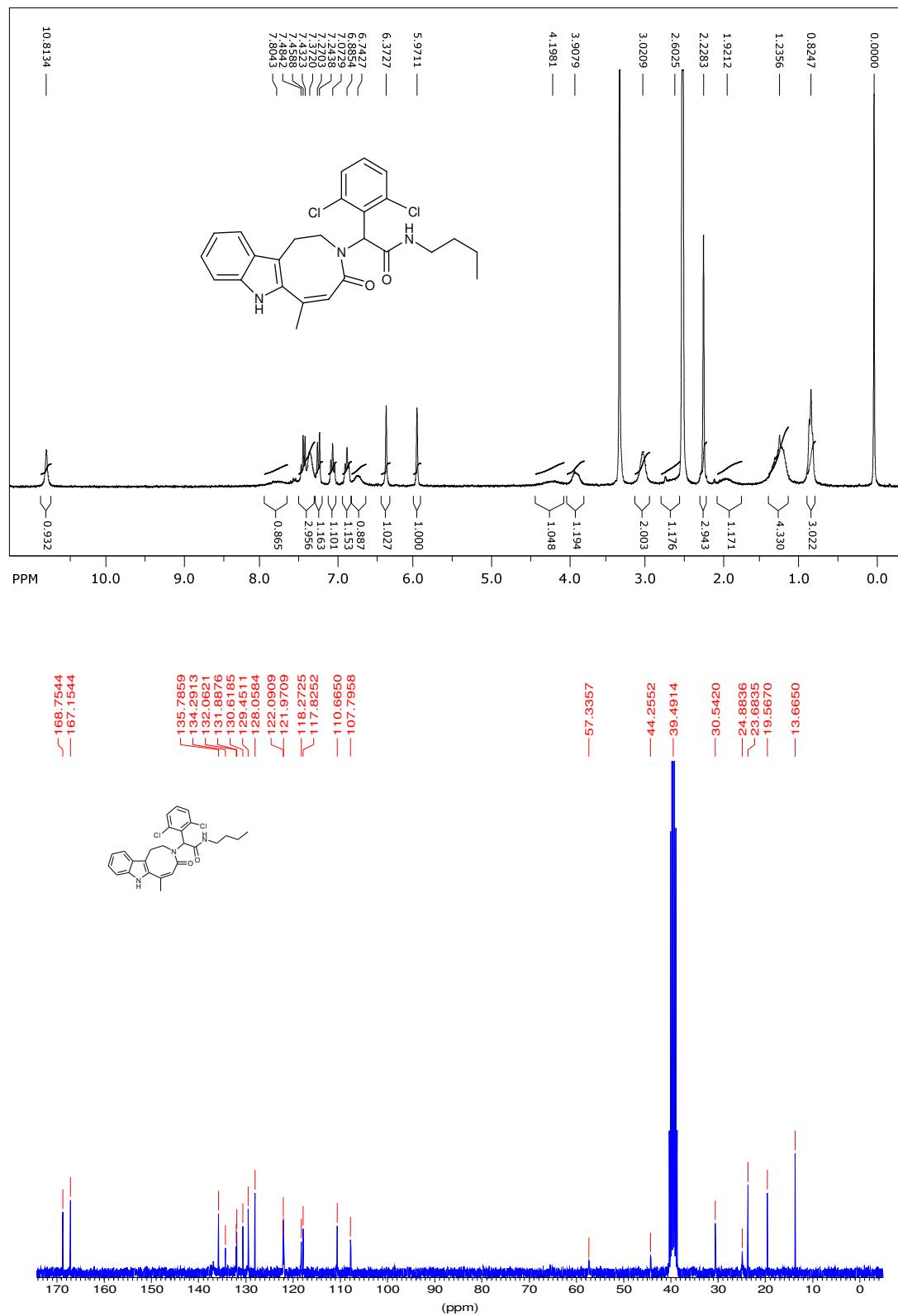
$^1\text{H}$  NMR (300 MHz, DMSO-d<sub>6</sub>) and  $^{13}\text{C}$  NMR (75 MHz, CDCl<sub>3</sub>) of compound **6k**
