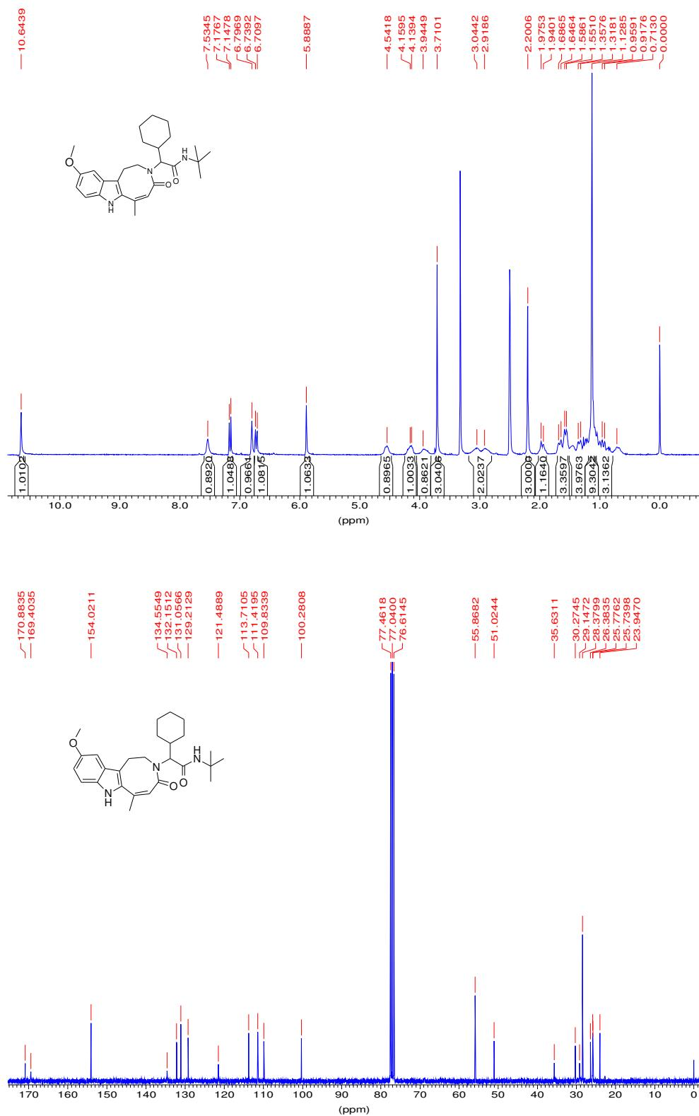
$^1\text{H}$  NMR and  $^{13}\text{C}$  NMR of compound **6m** (300 MHz,  $\text{CDCl}_3$ )
