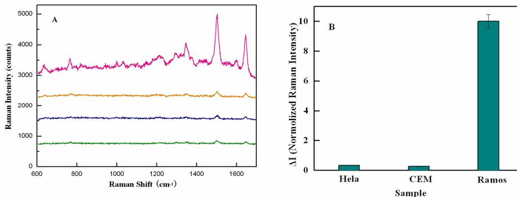
**Figure S6.** Specificity for the detection of Ramos cell against CEM and Hela. Numbers of Hela, CEM and Ramos cells all 50 cells, SERS spectra (A) and (B) normalized Raman intensity. The blank was subtracted for each value.
