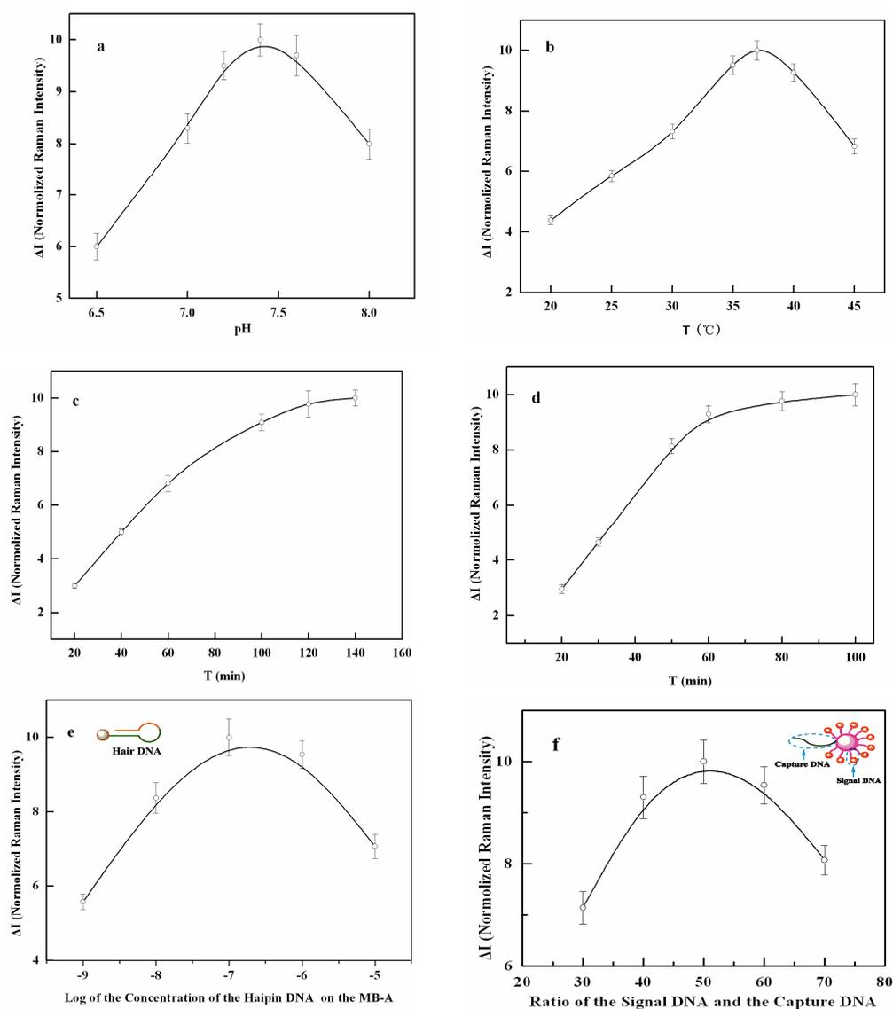
**Figure S3.** (a). Effect of the temperature and (b) pH of the cycle reaction. on the  $\Delta I$  signal. (c). Effect of optimization of the time of the DNA machine operation and (d) RCA reaction on the  $\Delta I$  signal. (e). Effect of the concentration of the hairpin DNA immobilized on the MB on the  $\Delta I$  signal. (f). Effect of the proportion of the signal probes and the capture probe immobilized on the Au NP on the  $\Delta I$  signal. Target DNA1 concentration,  $10^{-14}$
