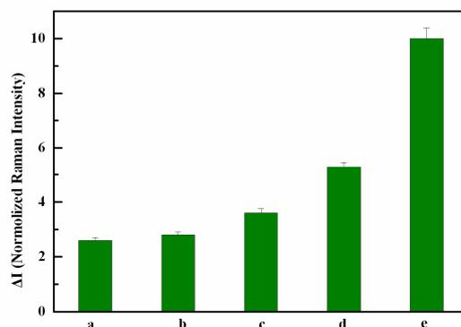
**Figure S2.** SERS spectra obtained from DNA machine with completing cycle 1 and RCA reaction with the prolong time: 2 min (a), 5 min (b), 10 min (c), 20 min (d), with completing cycle 1 and cycle 2 and RCA reaction (e), target DNA 1 concentration,  $10^{-14}$  M.
