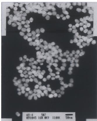
**Figure S4.** The TEM of Au NPs (~20 nm).
