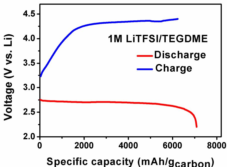
**Fig. S9** Discharge and charge curve of Li-O<sub>2</sub> battery with TEGDME based electrolyte
