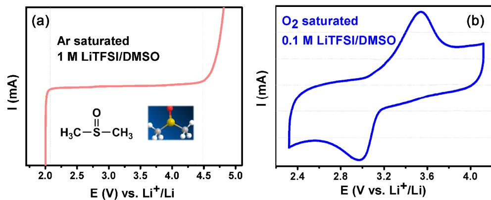
**Fig. S1** (a) Electrochemical window (versus Li<sup>+</sup>/Li) of 1 M LiTFSI/DMSO electrolyte under Ar atmosphere, and (b) Cyclic voltammogram of 0.1 M LiTFSI/DMSO under O<sub>2</sub> atmosphere.
