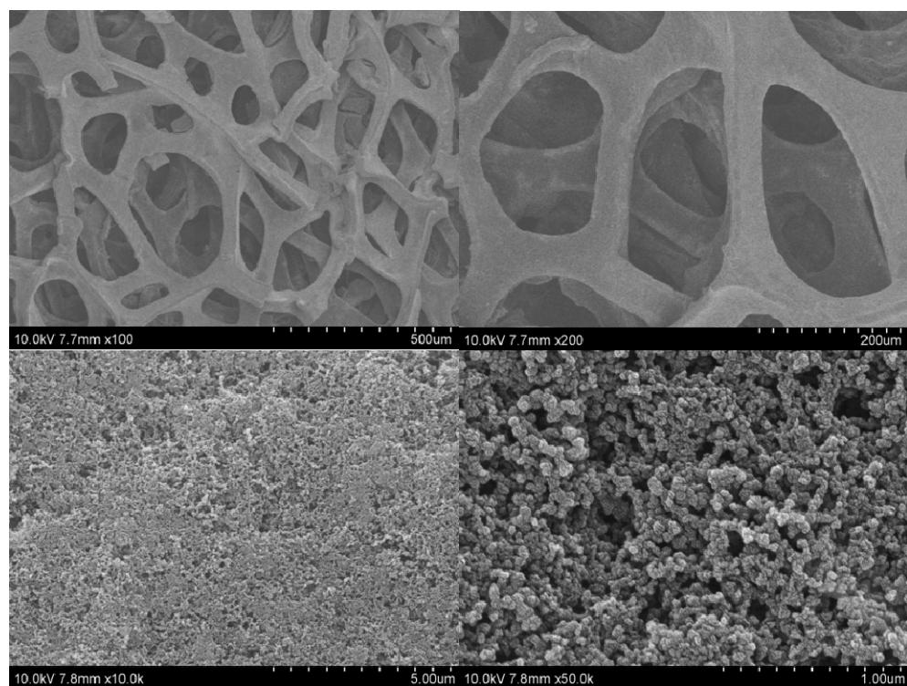
**Fig. S5** SEM images of fresh O<sub>2</sub> electrode with KB carbon on Ni foam.
