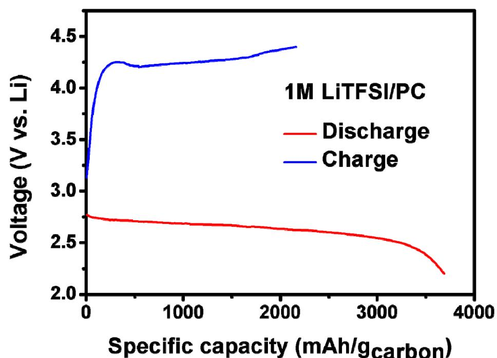
**Fig. S8** Discharge and charge curve of Li-O<sub>2</sub> battery with PC based electrolyte.
