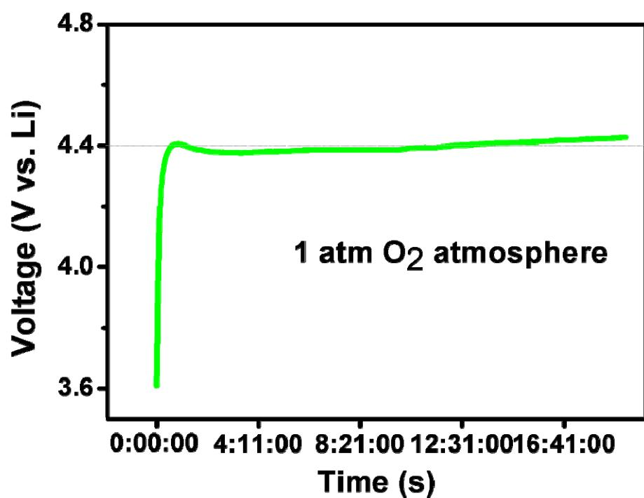
**Fig. S3** Charge curve of DMSO based electrolyte under 1 atm O<sub>2</sub> pressure.
