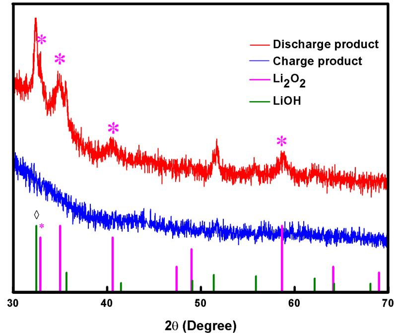
**Fig. S7** XRD spectra of discharged and charged cathode.
