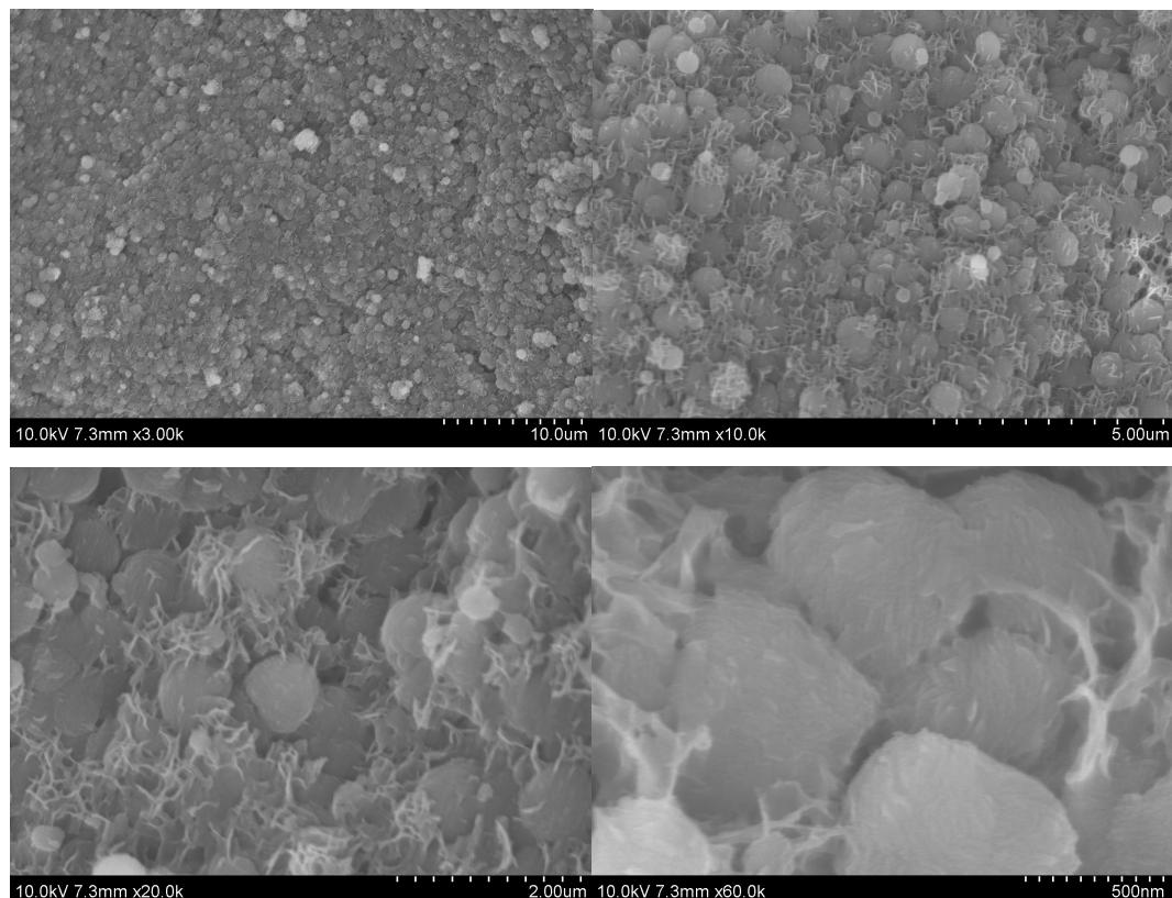
**Fig. S6** SEM images of O<sub>2</sub> electrode after discharge on KB carbon based cathode.
