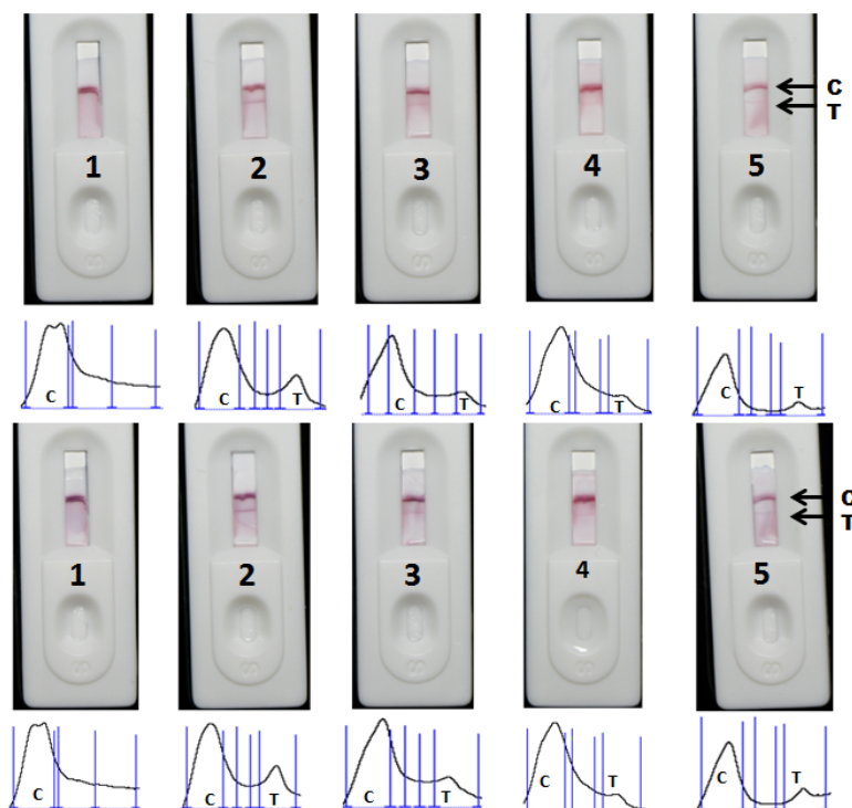
Figure S5: Images of test strips and peak areas using LNA-AuNP signaling probes specific for E. coli O157:H7 target detection, before (A) and after (B) signal amplification. Target DNA ET was added at a concentration of 0, 3.13, 1.56, 0.78 or 0.39 nM (strips 1-5, respectively). "C" and "T" denotes control and test lines respectively.
