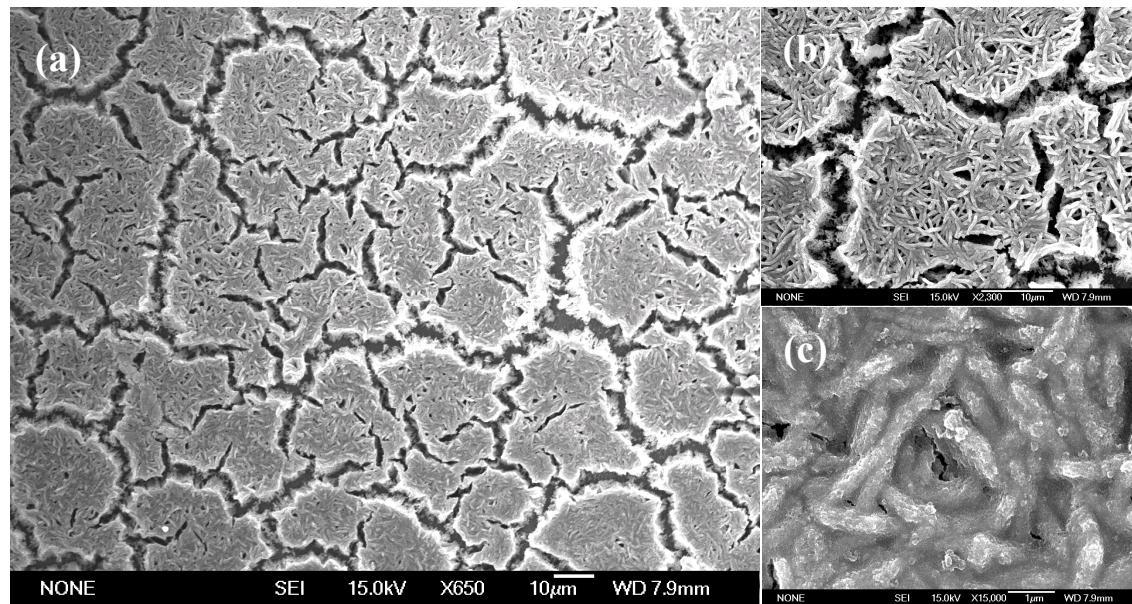
**Fig. S6** SEM observations towards the Ni NFs/MnO<sub>2</sub> hybrid electrode after 120 programmed discharge-charge cycles.
