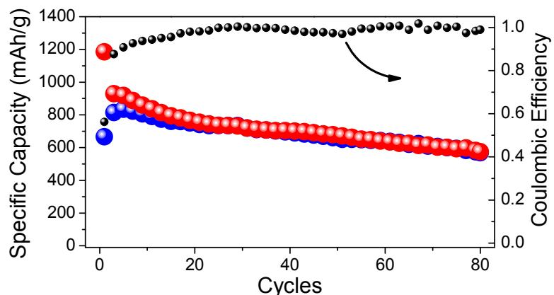
**Fig. S7** Cycling performance for the Ni NFs/MnO<sub>2</sub> hybrid electrode at a current density of 369 mA/g.
