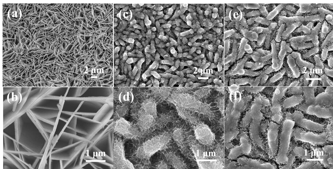
**Fig. S3** SEM observations of the evolution of the Ni NFs/MnO<sub>2</sub> hybrid electrode: (a-b) nullaginite NAs; (c-d) MnO<sub>2</sub>/nullaginite NAs; (e-f) MnO<sub>2</sub>/Ni NAs.
