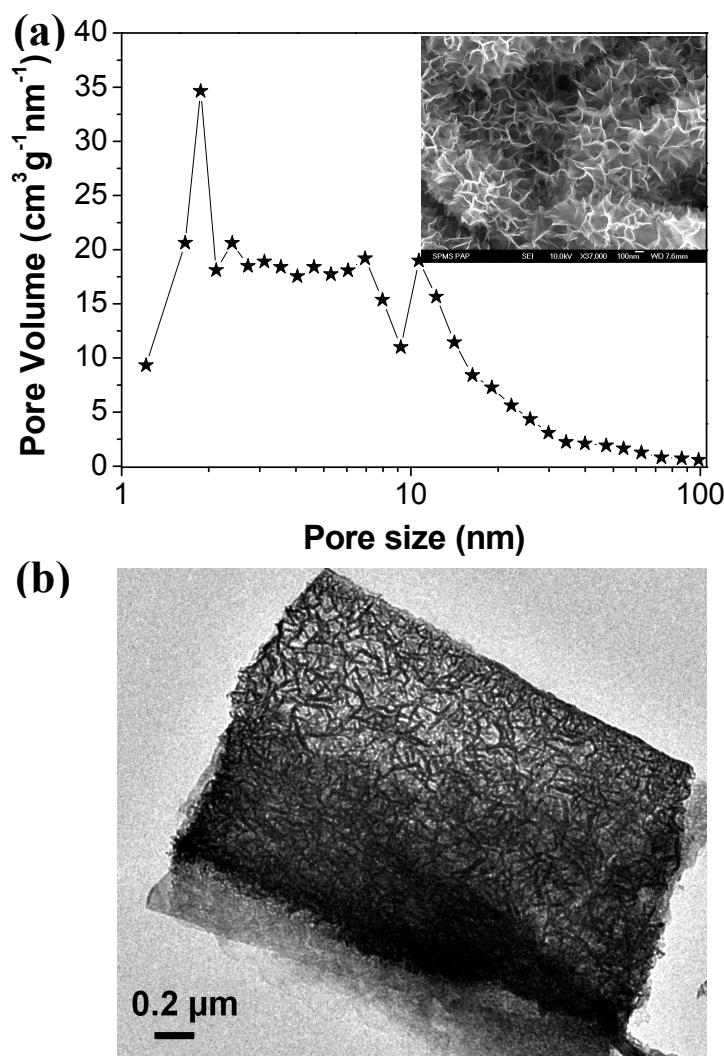
**Fig. S1** (a) The pore size distribution of the  $\text{MnO}_2$  nanoflakes. The inset SEM image shows the  $\text{MnO}_2$  nanoflakes are interconnected with each other. (b) TEM image of the Ni/ $\text{MnO}_2$  hybrid.
