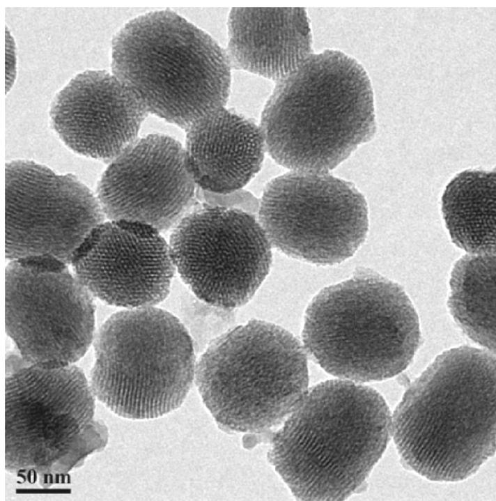
**Figure S3.** TEM of ALK-MSN showed formation of well-ordered two-dimensional hexagonal mesoporous particles with a spherical morphology having particle size of  $90 \pm 10$  nm
