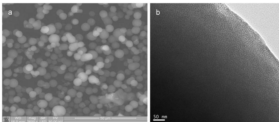
**Figure S2.** (a) SEM and (b) TEM images of AZP-SBA showed formation of spherical morphology particles with particle size of 5-8 μm and disordered mesoporous structure.<sup>9</sup>
