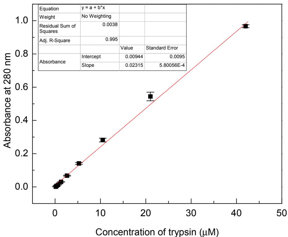
**Figure S11.** Calibration curve for trypsin in 10% PEG solution prepared in 50 mM, pH 8 tris buffer
