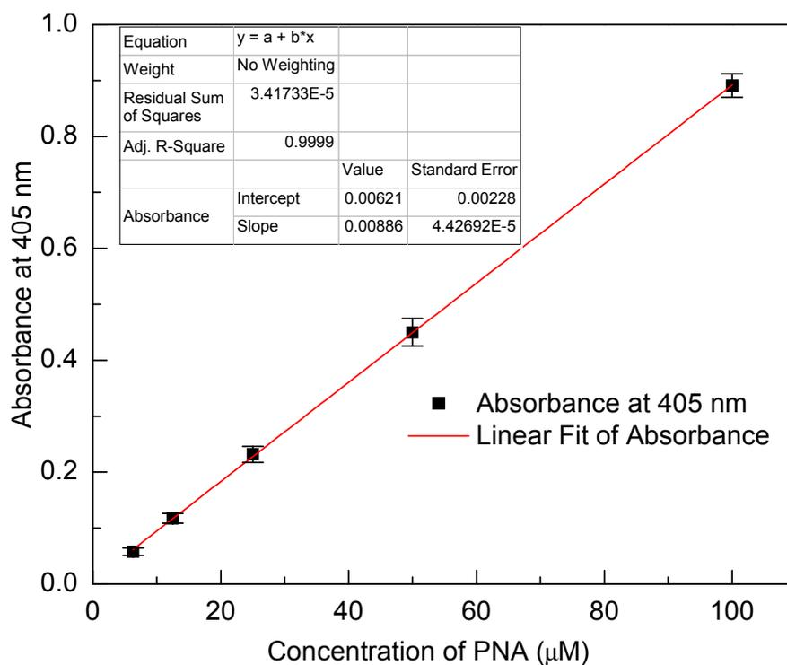
**Figure S12.** Calibration curve for p-nitroaniline (PNA) in 50 mM, pH 8 tris buffer.
