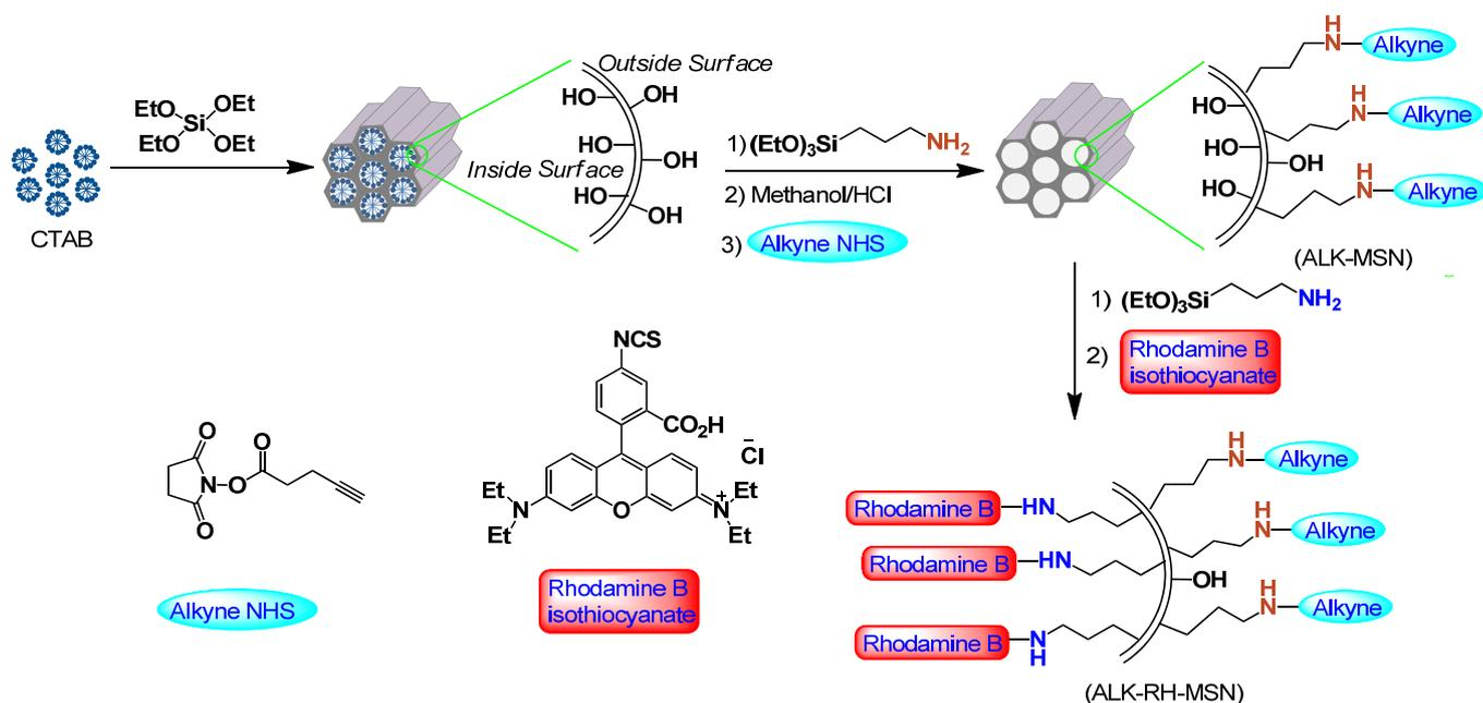
**Scheme S1.** Synthesis of outer surface alkyne functionalized and inner surface rhodamine B functionalized MSNs
