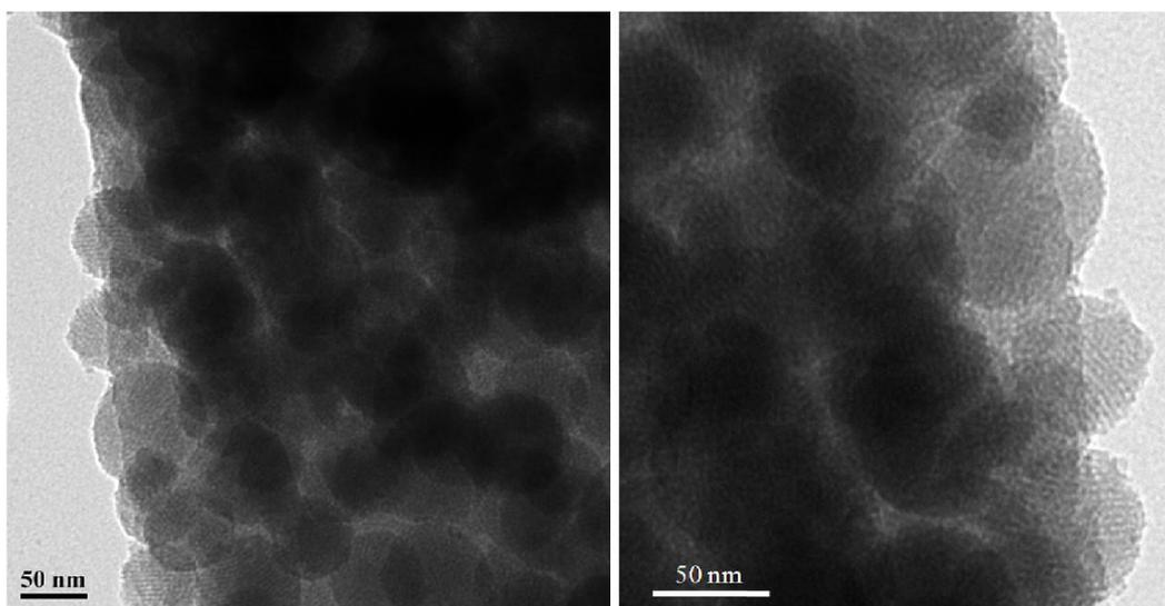
**Figure S4.** TEM images of Trypsin-SBA-MSN showing formation of hierarchical mesoporous structure
