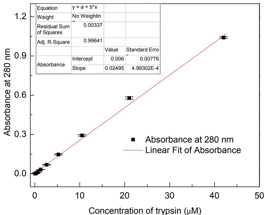
**Figure S10.** Calibration curve for trypsin in 100 mM, pH 7 phosphate buffer
