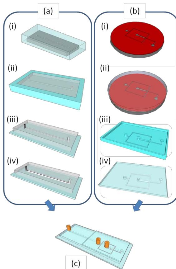
**Figure S1.** Schematic of the hybrid device fabrication, (a) LC separation channel in the first layer (i) PDMS casting from the master mould (ii) separation of the PDMS mould, TPE pouring then semi-curing at 60 °C (iii) bonding on PET substrate and full-curing at 76 °C (iv) packing the channel by C18 beads, (b) droplet generation channel in the second layer (i) SU-8 master mould (ii) PDMS casting (iii) bonding on PET substrate and full-curing at 76 °C (iv) packing the channel by C18 beads
