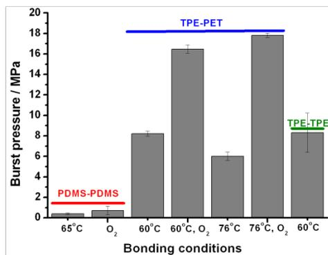
Figure S3. Burst pressure test as a function of bonding conditions and device materials
