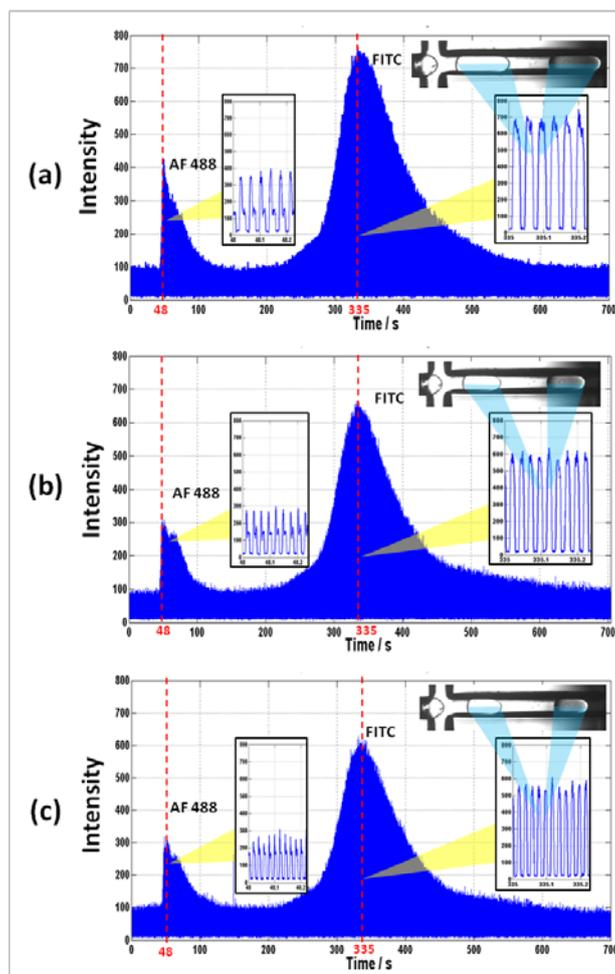
Figure S4. Chromatograms of separated dyes (AF488 and FITC) after compartmentalisation with (a) 27 Hz droplet generation (50  $\mu$ l/min running buffer-50  $\mu$ l/min oil) (b) 39 Hz droplet generation (50  $\mu$ l/min running buffer-75  $\mu$ l/min oil) and (c) 50 Hz droplet generation (50  $\mu$ l/min running buffer-100  $\mu$ l/min oil)
