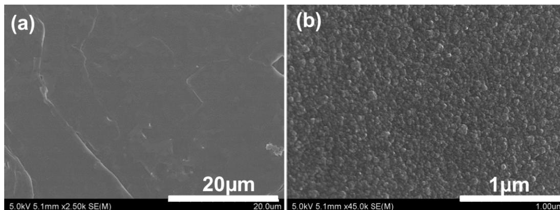
Fig. S1 SEM images of the PPy film prepared with  $\text{FeCl}_3$  as the oxidant and PTS as the dopant. (a) Low magnification; (b) high magnification. Synthetic conditions:  $[\text{FeCl}_3]=[\text{PTS}]=0.36\text{ M}$ ,  $[\text{Py}]=0.18\text{ M}$ .
