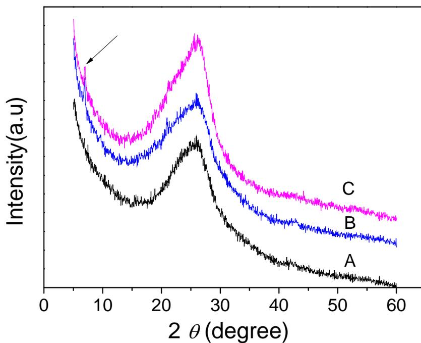
Fig. S2 XRD patterns of the PPy films prepared with different  $n(\text{PTS})/n(\text{Py})$ . The synthetic conditions are:  $[\text{Py}]=0.18\text{ M}$ ,  $[\text{FeCl}_3]=0.36\text{ M}$ , and the  $n(\text{PTS})/n(\text{Py})$  for the samples are 0/1(A), 4/1 (B) and 2/1 (C).
