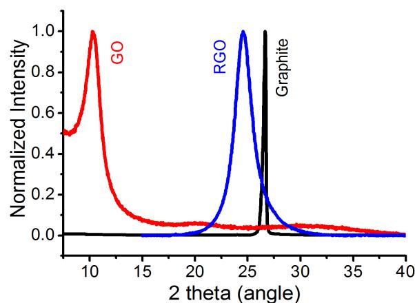
**Fig. S2.** XRD data of GO, control rGO and Graphite.
