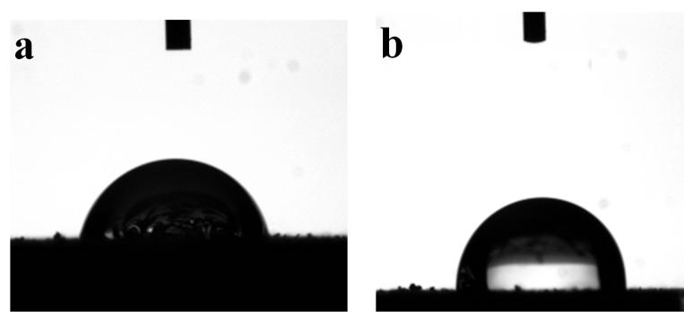
**Fig. S4.** (a) Contact angle images of 1<sup>st</sup> product ( $73^\circ$ ). (b) Contact angle images of 2<sup>nd</sup> product ( $86^\circ$ ).
