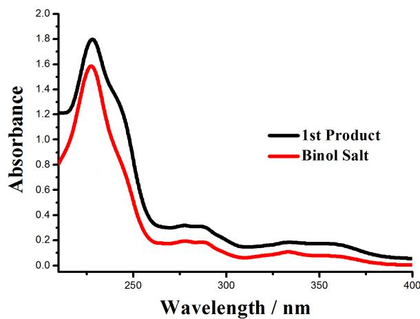
**Fig. S3.** UV-Vis spectra of 1<sup>st</sup> product (0.04 mg/mL) and Binol Salt (0.025 mg/mL).
