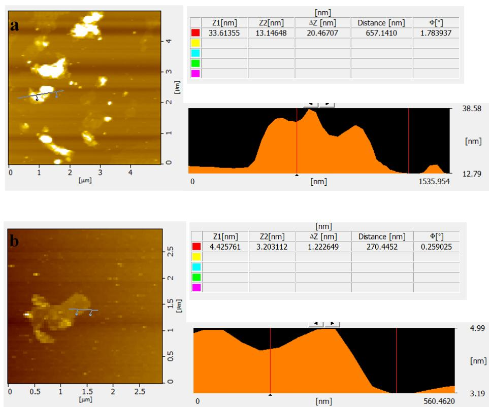
**Fig. S5.** (a) AFM image of 1<sup>st</sup> product (20 nm height). (b) AFM image of 2<sup>nd</sup> product (1.2 nm height).
