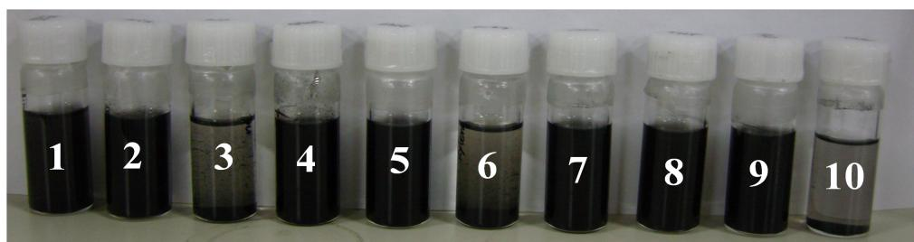
**Fig. S6.** Solubility Test of 1<sup>st</sup> product in a variety of solvents prepared by 2 h sonication (1mg/mL). Photographs of 1<sup>st</sup> product dispersed were taken 1 week after preparation, 1: Isopropyl alcohol; 2: Acetonitrile; 3: Toluene; 4: Dimethylsulfoxide; 5: Dimethylformamide; 6: *p*-Xylene; 7: N-Methylpyrrolidone; 8: Tetrahydrofuran; 9: Ethanol; 10: Dichloromethane.
