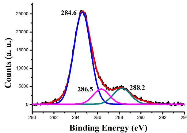
**Fig. S1.** High-resolution C1s XPS spectra of binol salt.
