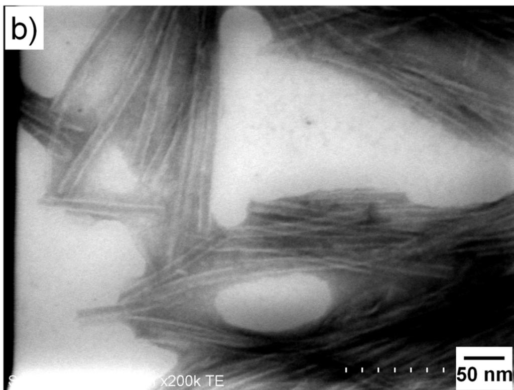
**Figure S11** STEM images of CDDP@ONT after the release experiment in a) HBS and b) HEPES buffer. In a) Red arrows: ONTs; Blue arrows: Nanofibers.
