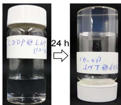
**Figure S6** Formation of hydrogel from mixture solution of 1-Na and CDDP(molar ratio of 1/1) .
