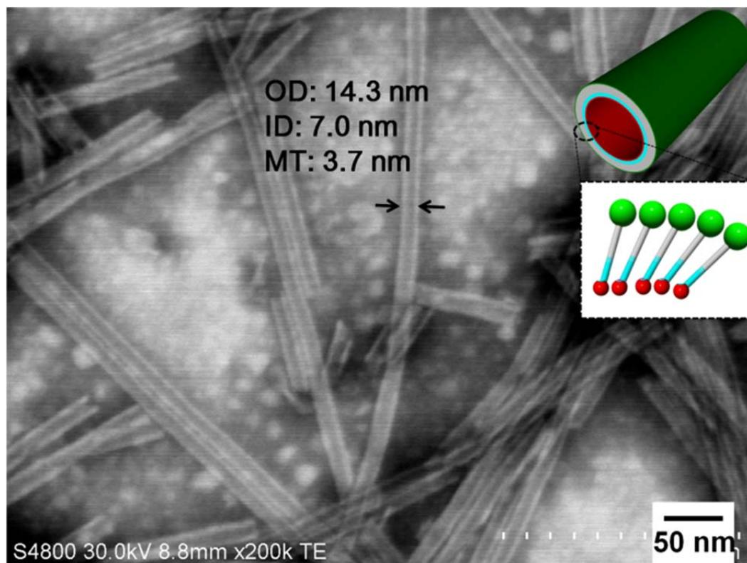
**Figure S9** STEM image of bare ONT self-assembled from 1 alone. This bare ONT was prepared from
