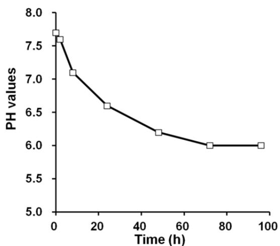
**Figure S8** Time dependent pH shift of the mixture solution containing 1-Na and CDDP (molar ratio of 1/1).
