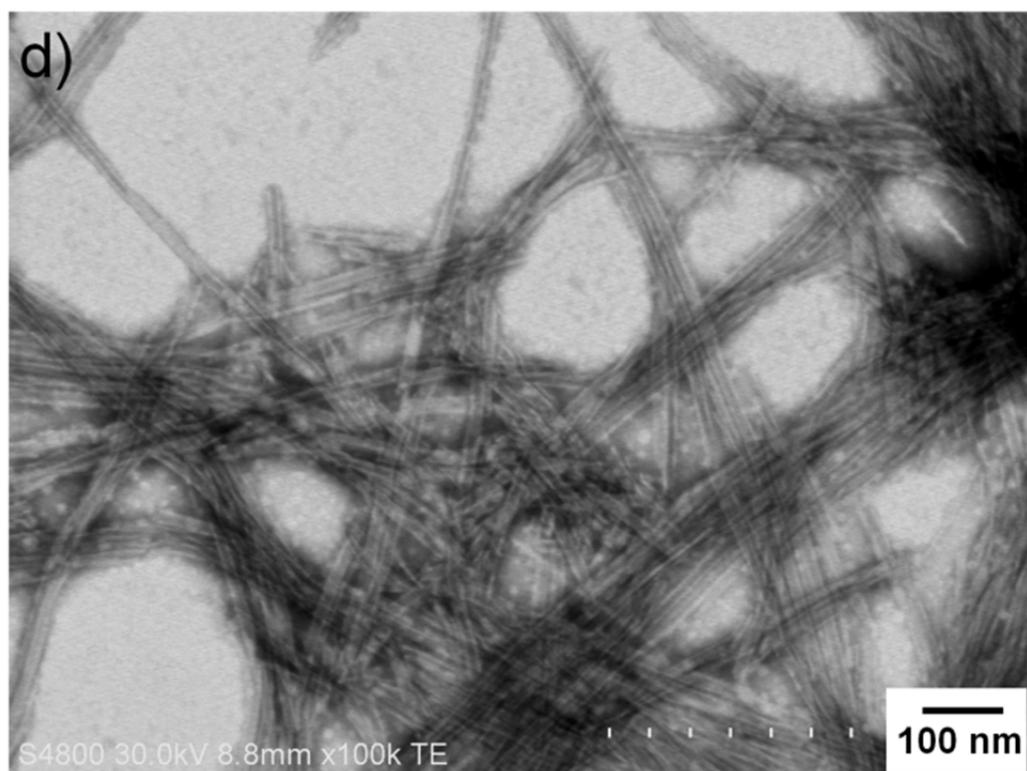
**Figure S5** Time-dependent STEM images of mixture solution containing **1**-Na and CDDP (molar ratio of 1/1) upon drying on carbon grids and staining with 2%-phosphotungstate. **a)** 2 h; **b)** 8 h; **c)** 24 h; **d)** 48 h incubation time. Red arrows: ONTs; Blue arrows: Nanofibers.
