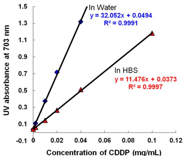
**Figure S2** Calibration curves of CDDP in water and HBS buffer. The calibration curves were linear with correlation coefficients higher than 0.999 over the concentration range of 2–100  $\mu\text{g/mL}$ . The relative lower detection sensitivity in HBS buffer might attribute to the ions in HBS buffer.
