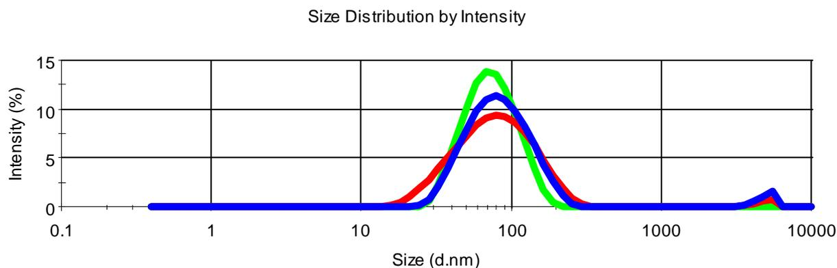
**Figure S3** Dynamic light scattering of **1**-Na dispersion in water (2 mg/mL). Green line, at room temperature; Blue line, at 4 °C; and Red line, at 50 °C.
