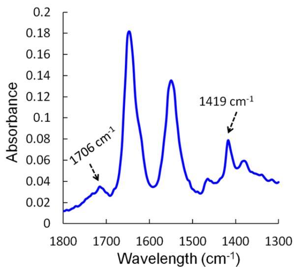
**Figure S7** IR spectra of **1** as acidic form. The broad peak around  $1706\text{ cm}^{-1}$  is assigned to the  $-\text{CO}_2\text{H}$  group, the peak of  $1419\text{ cm}^{-1}$  is assigned to the C–H deformation band of tetraglycines.
