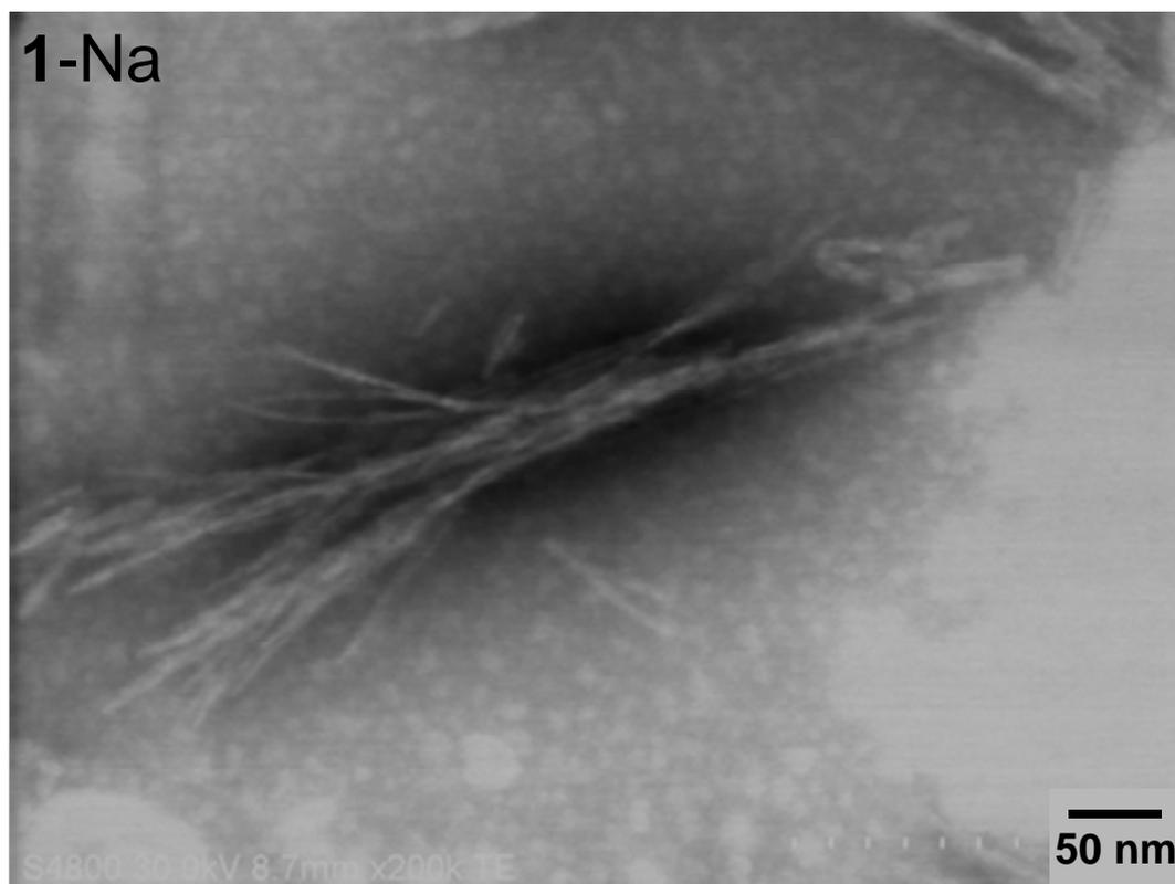
**Figure S4** Nanofibers obtained from **1-Na**. The sample solution was rapidly evaporated on a carbon grid and stained with 2%-phosphotungstate (pH 8).
