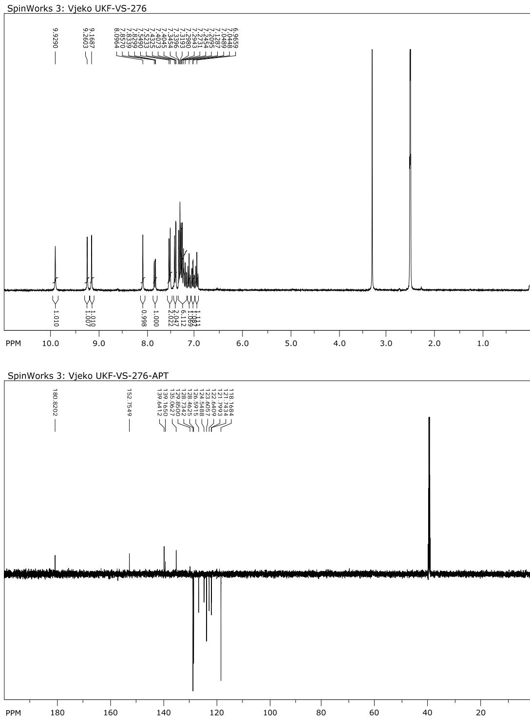
**Figure S22.**  $^1\text{H}$  and  $^{13}\text{C}$  NMR spectra of mixed urea-thiourea **2k**.
