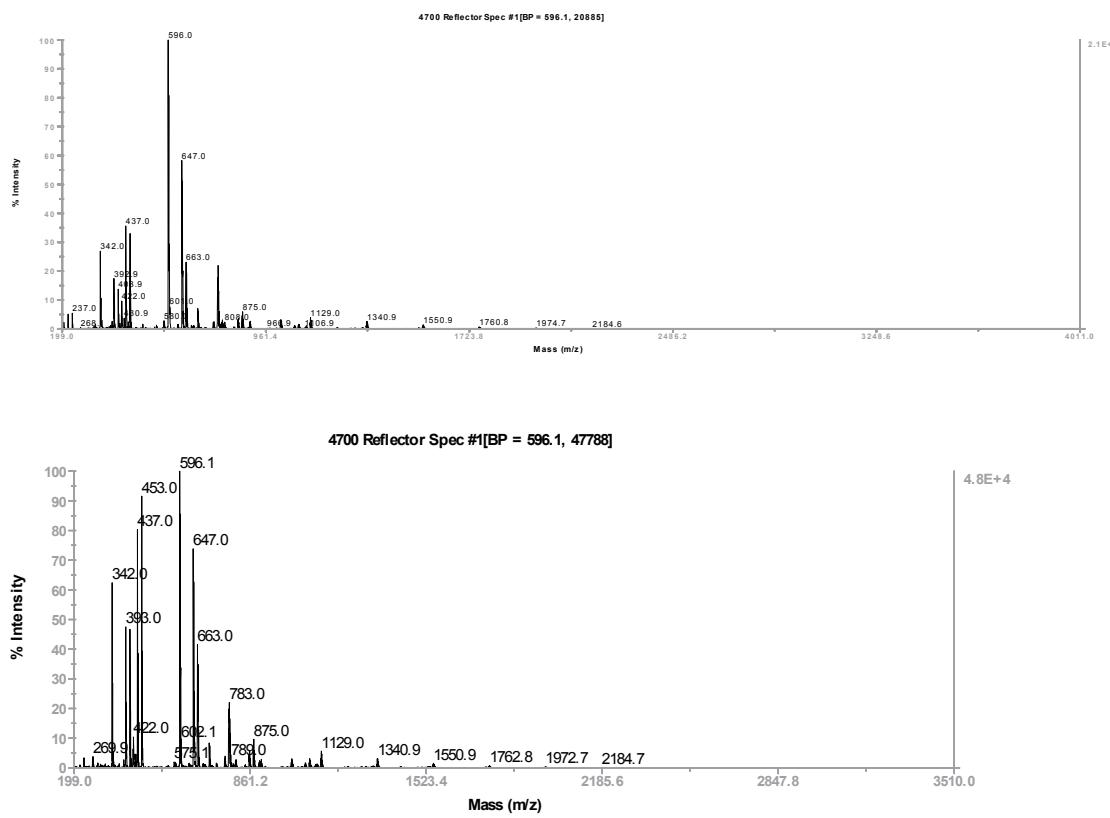
**Figure S3.** MALDI-TOF mass spectra for compounds **2** and **4**, pointing out their similar high degree of fragmentation in low molecular weight species in solution.
