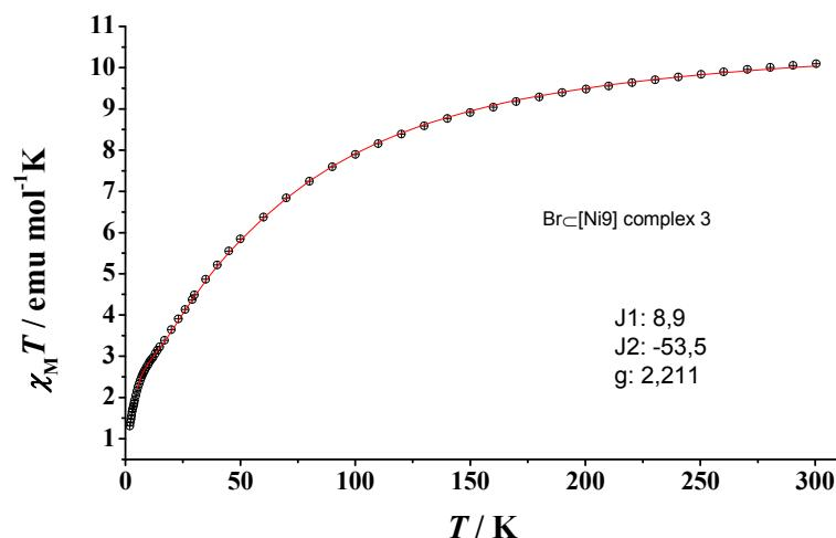
**Figure S4.**  $\chi_M T$  plot vs  $T$  for complex  $(\text{Br}) \subset [\text{Ni}_9(\text{dpt})_6(\text{pyC}\{\text{ph}\}\text{NO})_6(\text{N}_3)_9]\text{Br}_2$  (**4**). Shape and  $\chi_M T$  values are practically identical to compound **2** and it has not been included in Figure 5 for clarity. As can be expected from the ring structural data, the guest anion does not modify the magnetic properties.
