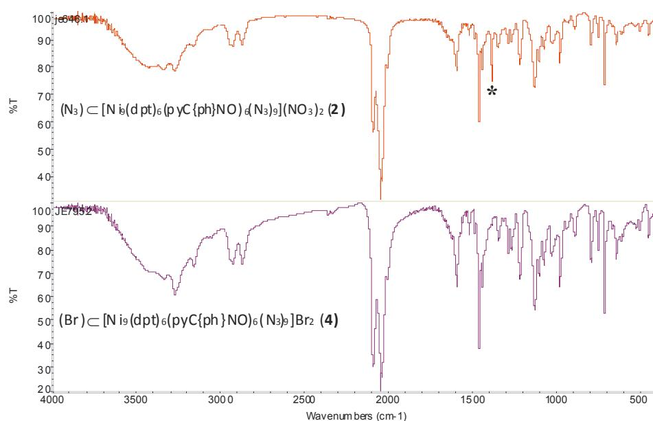
**Figure S1.** IR data for the reported complexes  $(\text{N}_3) \subset [\text{Ni}_9(\text{dpt})_6(\text{pyC}\{\text{ph}\}\text{NO})_6(\text{N}_3)_9](\text{NO}_3^-)_2$  (**2**), and  $(\text{Br}) \subset [\text{Ni}_9(\text{dpt})_6(\text{pyC}\{\text{ph}\}\text{NO})_6(\text{N}_3)_9]\text{Br}_2$  (**4**). As can be seen, the IR spectra do not differentiate the anionic guest. The only difference among these spectra is the anionic nitrate peak (\*).
