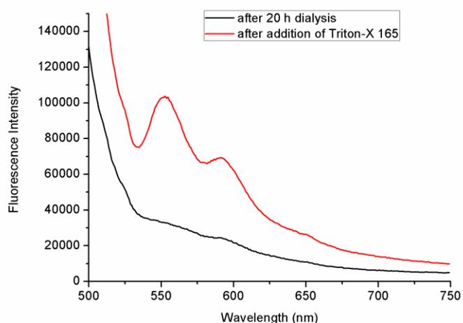
**Figure S8:** Fluorescence spectrum ( $\lambda_{\text{excitation}} = 479 \text{ nm}$ ) of a dialyzed solution of cavitand **8** and doxorubicin hydrochloride in water before (black) and after (red) addition of Triton X-165.
