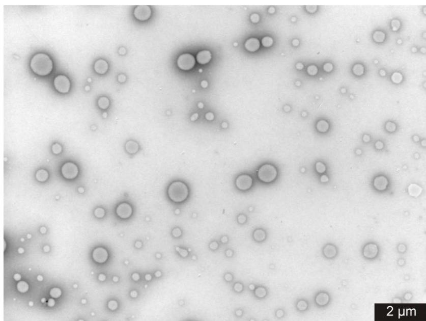
**Figure S6:** TEM image of vesicles of octa-TEG cavitand with short ethyl feet.
