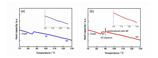
Fig. S1 DSC data of a mixture blended with 20 wt% of the chiral dopant (a) before and (b) after the UV irradiation at 90 °C during heating process.
