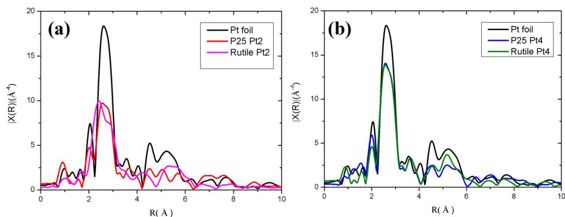
**Fig.S7** X-ray absorption studies: radial distribution functions of synthesized Pt/TiO<sub>2</sub>: using (NH<sub>4</sub>)<sub>2</sub>PtCl<sub>4</sub> as metal precursor, samples shown in Fig.1 (a); using H<sub>2</sub>PtCl<sub>6</sub>.6H<sub>2</sub>O as metal precursor, samples shown in Fig.S4 (b)
