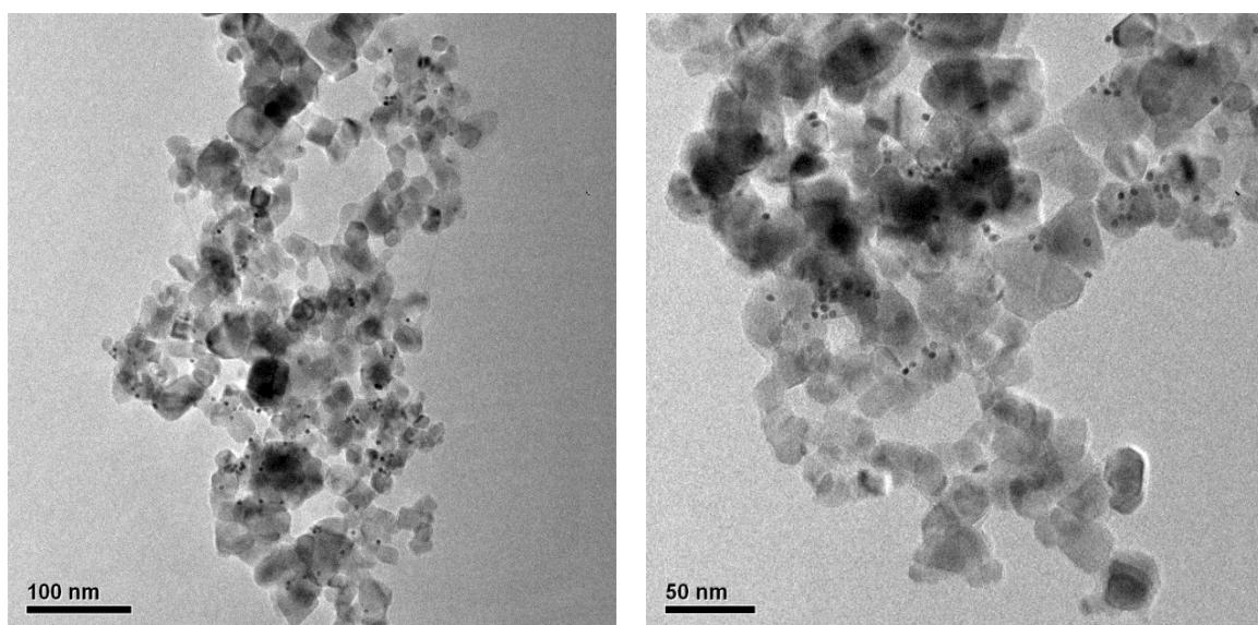
**Fig.S1** Pt/TiO<sub>2</sub> synthesized using colloidal deposition method
