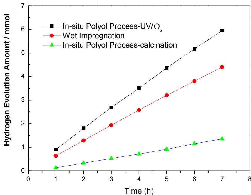
**Fig.S9** Photocatalysis hydrogen production amount from water/methanol for Pt/TiO<sub>2</sub> prepared by in-situ polyol process/UV-O<sub>2</sub> process, in-situ calcination process and wet impregnation respectively. In the calcination process, the catalysts were heated to 350 °C in air at heating rate of 2 °C/min and keeping at that temperature for 4 hours.
