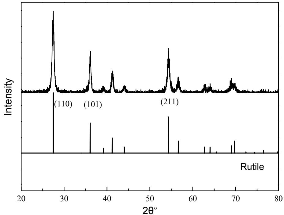
**Fig.S2** XRD pattern of rutile  $\text{TiO}_2$
