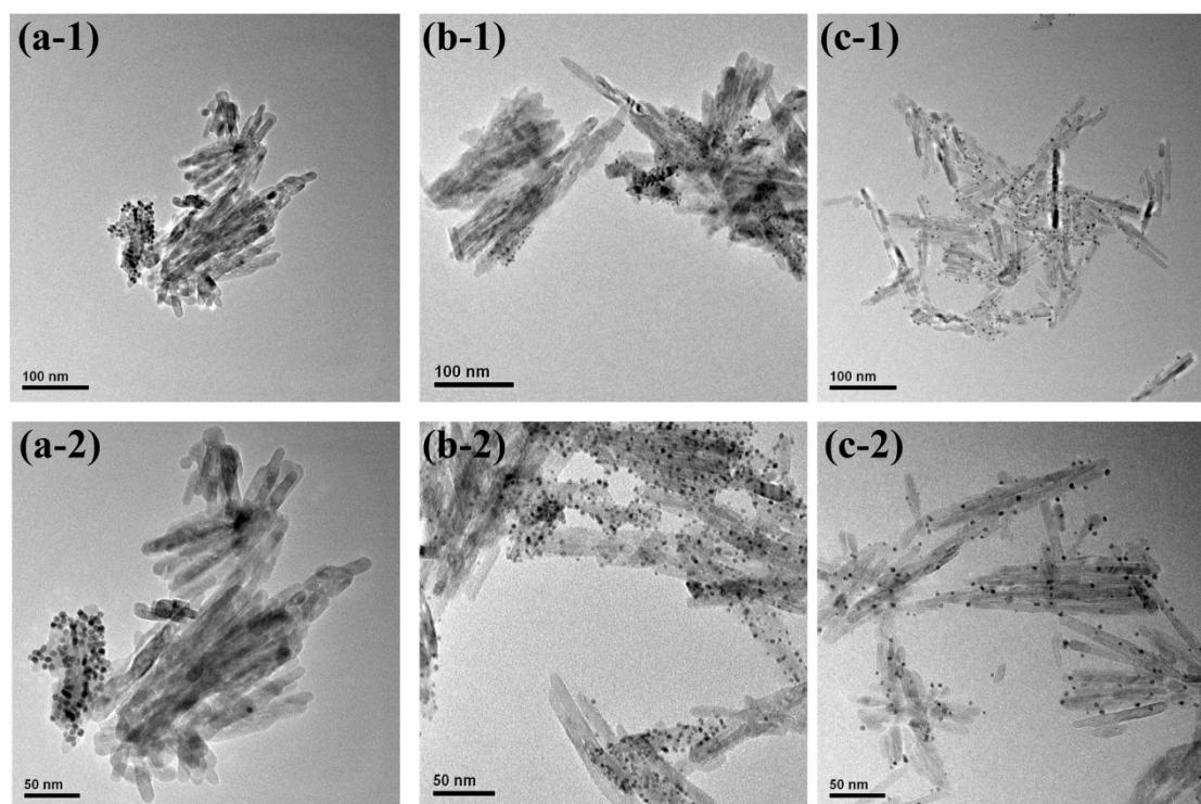
Fig.S3. Pt/TiO<sub>2</sub> synthesized without PVP (a-1,a-2), premixing TiO<sub>2</sub> and PVP at room temperature (b-1,b-2), premixing of PVP with TiO<sub>2</sub> in 60 °C and ultrasound for 30 minutes (c-1,c-2) using Pt (IV) salt ( $H_2PtCl_6 \cdot 6H_2O$ ) as metal salt precursor in ethylene glycol.
