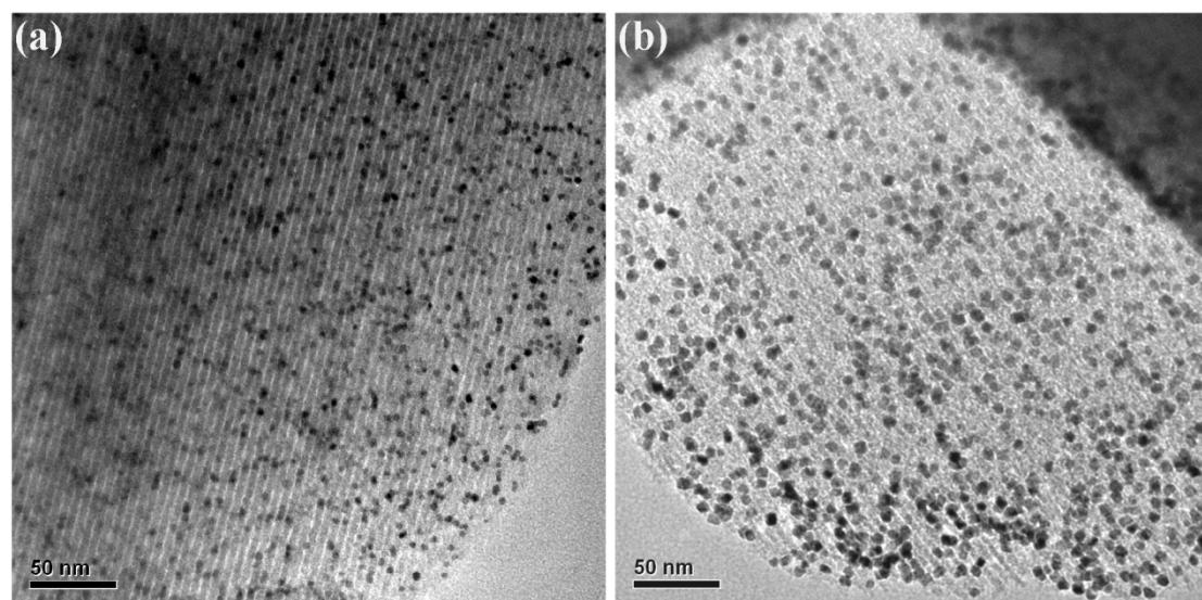
**Fig. S5** In situ synthesis Pt nanocrystals on  $\text{SiO}_2$  (a homemade SBA-15), using Pt(II) salt ( $(\text{NH}_4)_2\text{PtCl}_4$ ) (a) and Pt (□) salt ( $\text{H}_2\text{PtCl}_6 \cdot 6\text{H}_2\text{O}$ ) (b) as metal precursor respectively, together with PVP and TMABr
