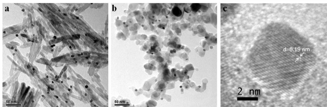
**Fig.S4** In-situ synthesis Pt nanocrystals on rutile TiO<sub>2</sub>(a) P25 TiO<sub>2</sub> (b) respectively , using Pt (IV) ( $\text{H}_2\text{PtCl}_6 \cdot 6\text{H}_2\text{O}$ ) salt as metal salt precursor in ethylene glycol together with PVP and TMABr, high resolution image of cubic Pt supported on TiO<sub>2</sub>(P25)(c)
