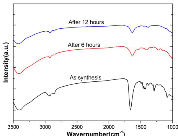
**Fig.S8** FT-IR spectra of Pt/TiO<sub>2</sub> under UV treatment at 0, 6, 12 hours under the irradiation of full-arc light
