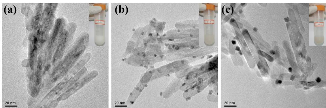
**Fig.S6** Pt/TiO<sub>2</sub> nanoparticles during the synthesis process: (a) 5 minutes (b) 6 minutes (c) 10 minutes
