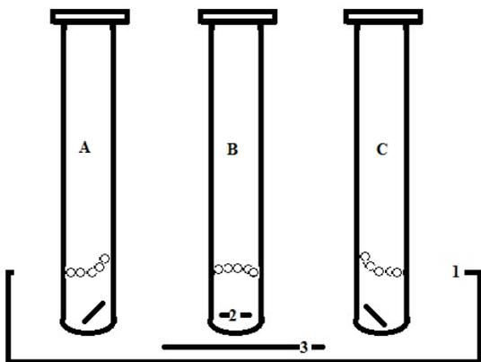
**Fig. S2.** Position of reaction tubes in heating bath. 1= Heating bath, 2= magnetic stirrer, 3= magnetic stirrer for heating bath. Diagram is not to measure.
