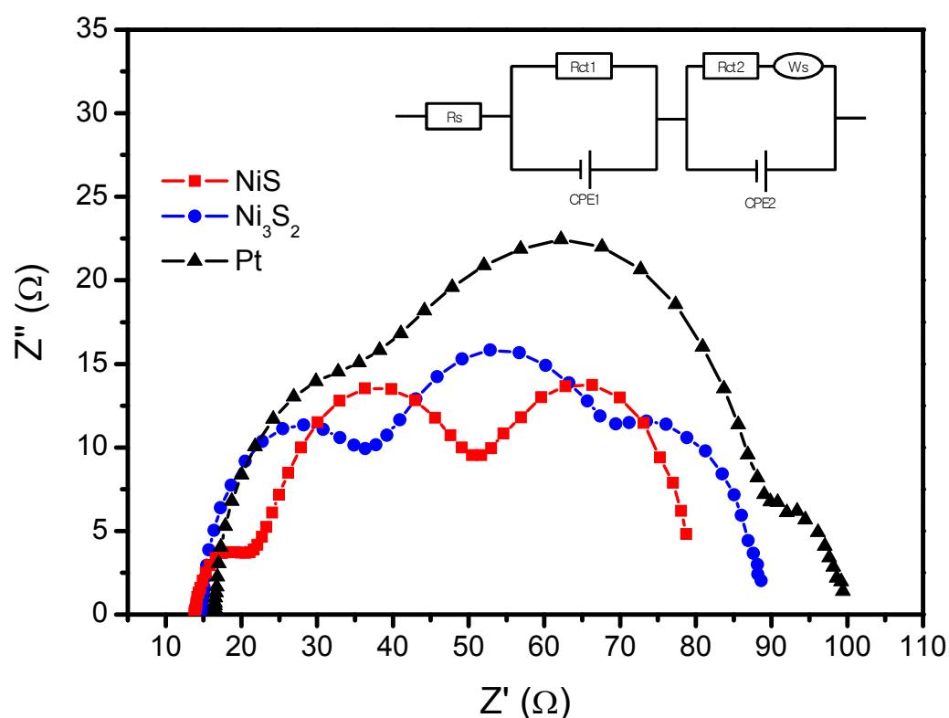
**Fig. S6.** (a) J-V curves and (b) Nyquist plots of qssDSSCs fabricated with two nickel sulfide counter electrodes using the spin-coating method.
