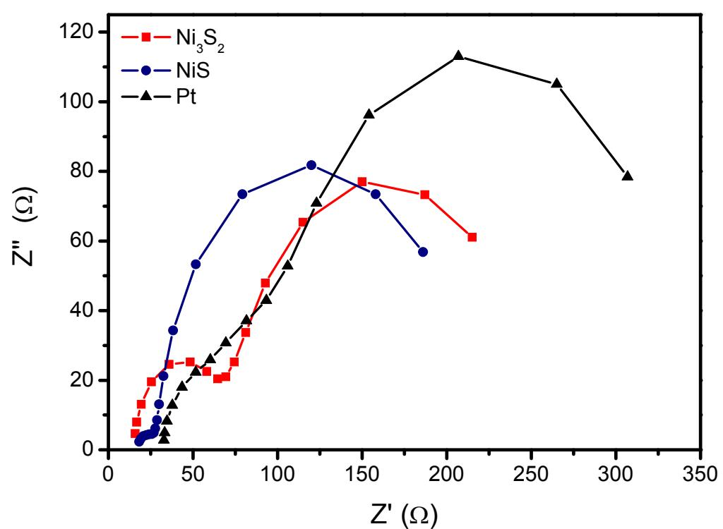
**Fig. S5.** Nyquist plots of the full qssDSSCs fabricated with different counter electrodes under 1 sun illumination with the frequency range from 0.01 Hz to 0.1 MHz. The inset shows the corresponding equivalent circuit.
