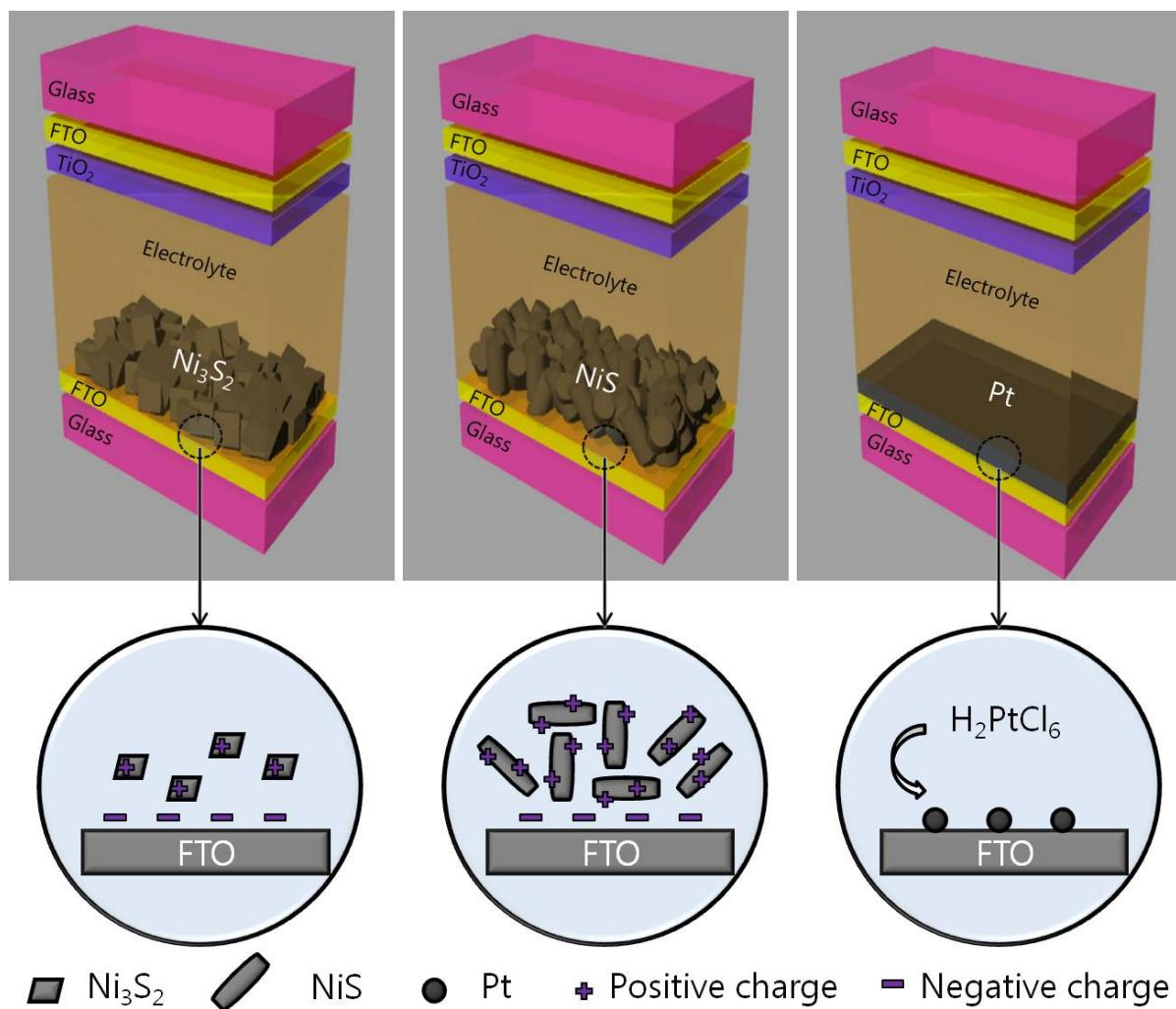
**Fig. S1.** Zeta potential of nickel sulfides in ethanol solution.
