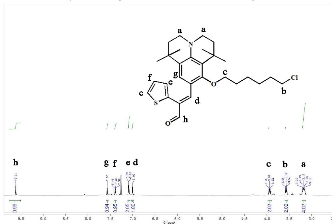
Figure 2  $^1\text{H}$  NMR spectra of compound **6**
