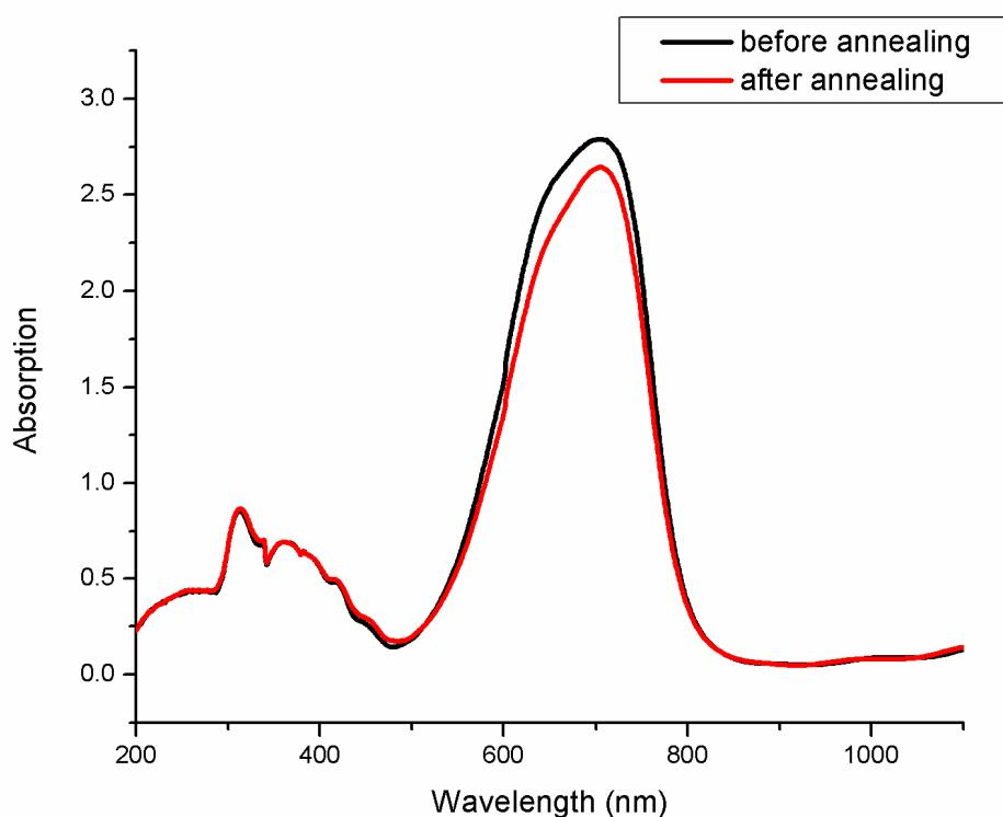
Figure 7 Absorption of EO film containing **WJ1** and N-phenylmaleimide before and after annealing
