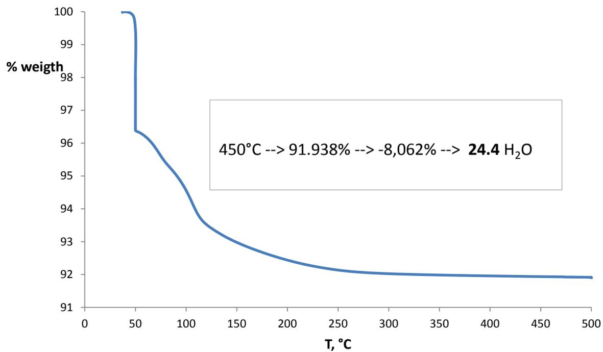
**Figure S3.** TGA analysis of crystals of **1**. The decrease of weight is due to loss of 24 hydration water molecules per molecule of **1**.
