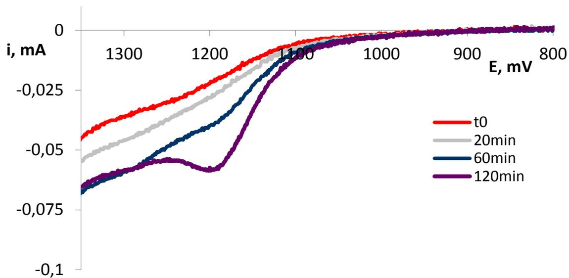
**Figure S4.** Time dependent CV scans of 2 mM **1** in 0.2 M borate buffer (pH 8).
