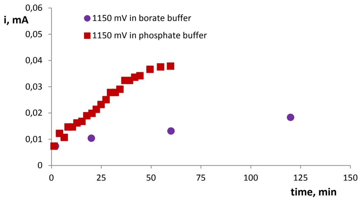
**Figure S5.** Plot of the anodic current at 1150 mV vs time observed in the CV of 2 mM **1** in 0.2 M phosphate (red squares) and borate (violet dots) buffers (pH 8).
