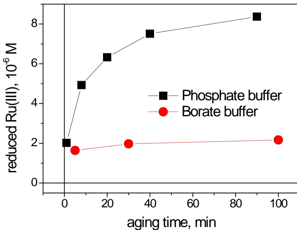
**Figure S7.** Amount of  $\text{Ru}(\text{bpy})_3^{3+}$  being reduced by  $5.0 \times 10^{-5}$  M **1** in laser flash photolysis ( $450 \mu\text{s}$  time window), as a function of the aging time of the solution used in 80 mM phosphate (black squares) and 80 mM borate (red dots) buffers (pH 8). The value of reduced Ru(III) corresponding to 100 min aging in borate buffer is obtained from kinetic traces not shown for clarity in Figure S6.
