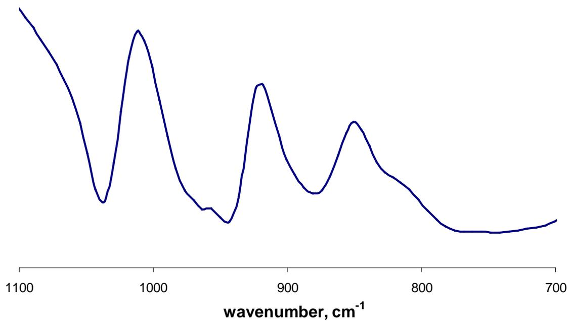
**Figure S1.** Infrared spectra of crystals of **1** (2% in KBr pellet).
