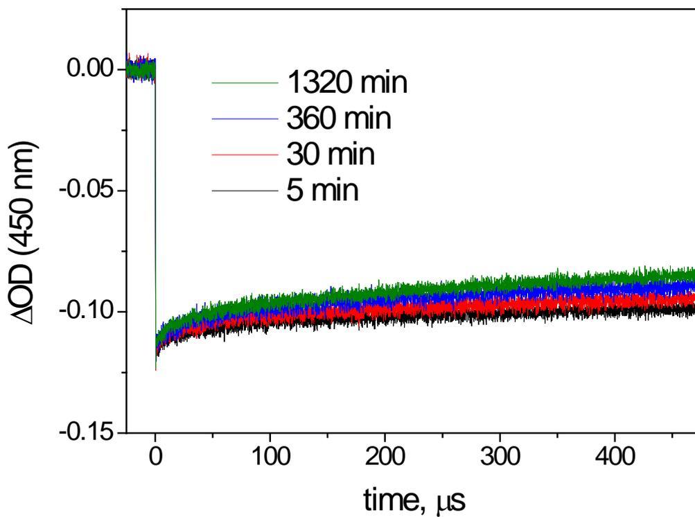
**Figure S6.** Hole scavenging kinetics measured using  $5.0 \times 10^{-5}$  M solutions of **1** of various aging time in 80 mM borate buffer (pH 8). Aging takes place in a  $10^{-3}$  M mother solution of **1** in 80 mM borate buffer (pH 8).
