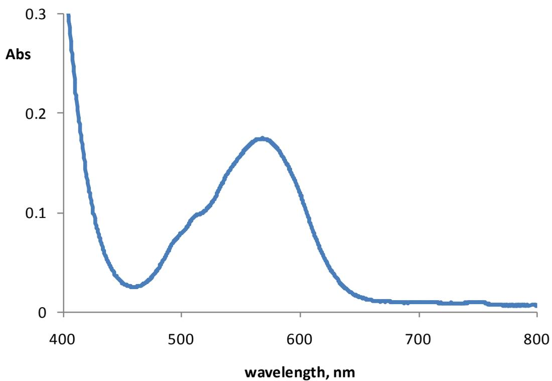
**Figure S2.** UV-vis spectra of a freshly prepared 1 mM solution of **1** in water.
