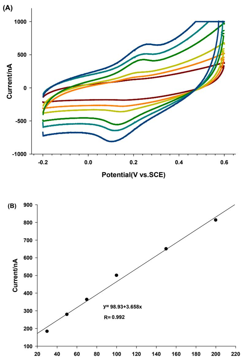
**Figure S2.** Cyclic voltammograms of the modified gold electrode at various scan rates, 30, 50, 70, 100, 150, 200 mV/s after addition of 5 mM L-histidine. (B) The plots of oxidation peak currents vs scan rate.
