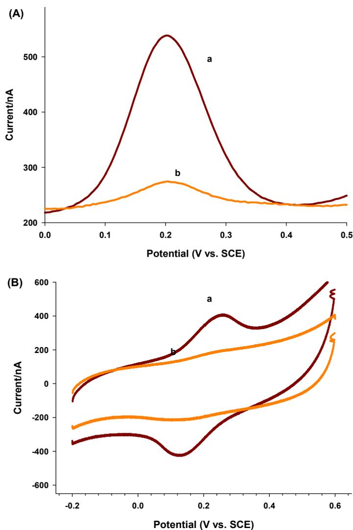
**Figure S5.** Electrochemical responses correspond to sensing systems recorded in 0.1 M KClO<sub>4</sub>. (A) Typical DPV curves of the sensor in response to 5 mM (line a) and 0 mM (line b) L-histidine, respectively. (B) The cyclic voltammograms a and b correspond to lines a and b in (A), respectively. Potential scanning rate is 100 mV/s.
