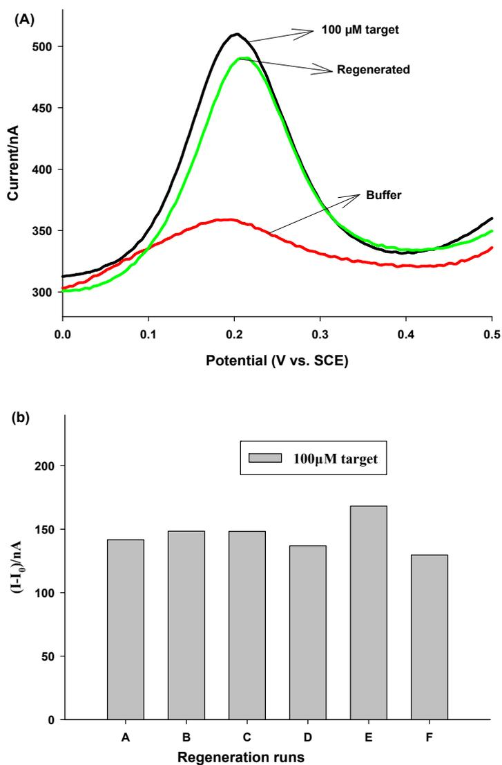
**Figure S6.** Typical DPV curves of the sensor in response to 100 μM and 0 μM L-histidine, and the current response after regenerated (A). The sensor shows no significant degradation after 6 cycles of use and regeneration (B).  $I$  and  $I_0$  represented the DPV peak current in the presence of and absence of 100 μM target.
