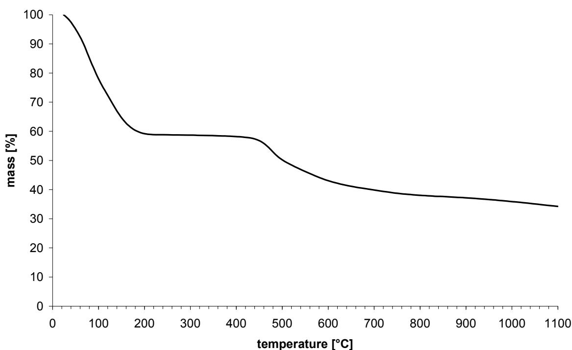
**Figure S5:** Thermogravimetric analysis of cage compound **5**.
