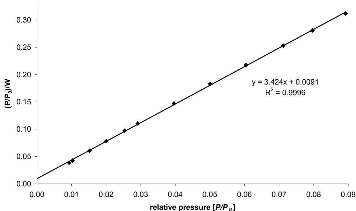
**Figure S7:** Langmuir-plot for [4+6] cage compound 5.
