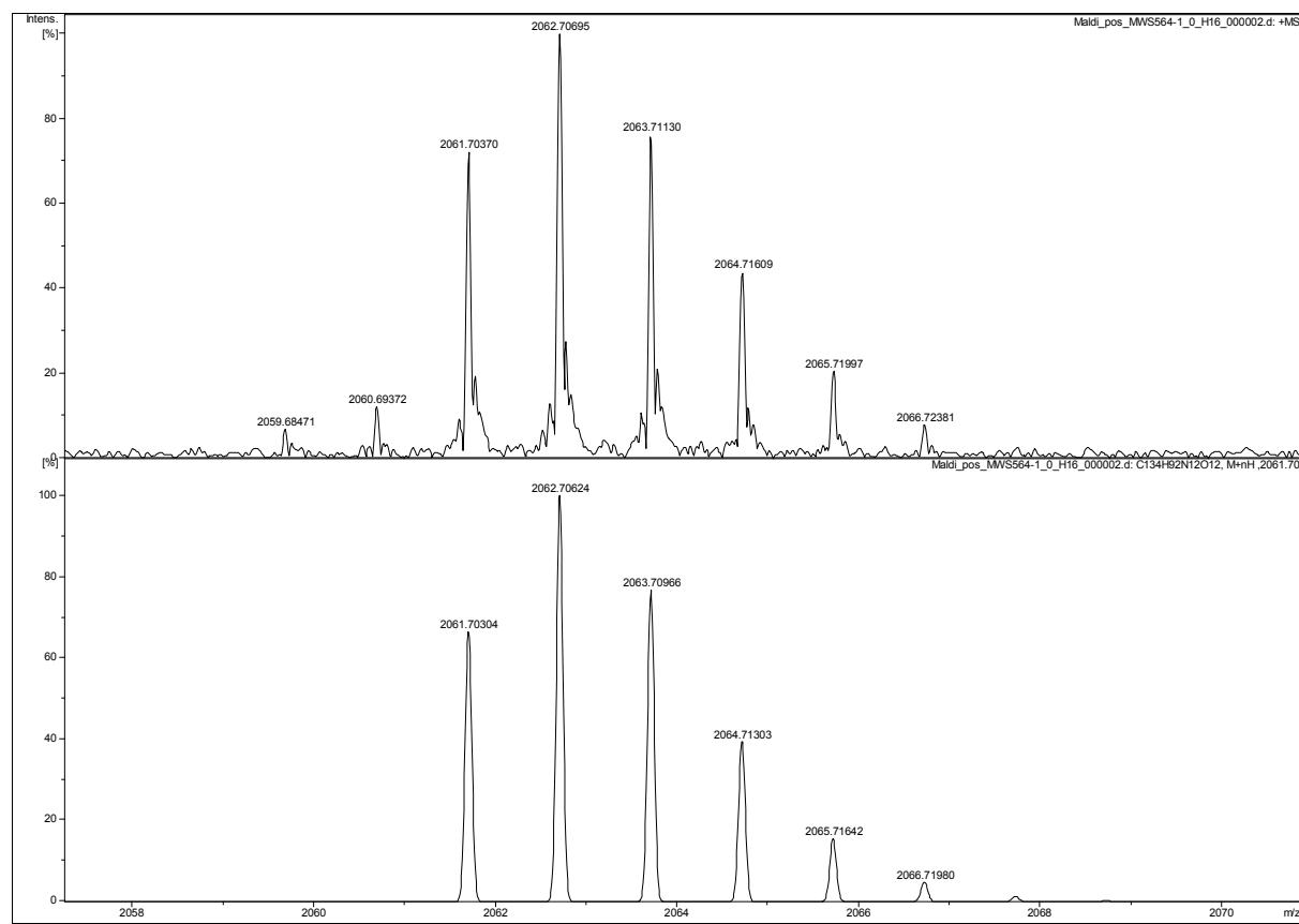
**Figure S4:** HR-MALDI mass spectrum of cage compound **5**. Top: zoom in section of the basis; bottom: calculated pattern.
