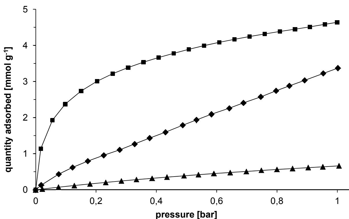
**Figure S8:** Gas adsorption isotherms for H<sub>2</sub> (squares, 77 K), CO<sub>2</sub> (diamonds, 273 K) and CH<sub>4</sub> (triangles, 273 K) for cage compound 5.
