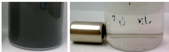
Figure S3. The rGO-Fe(0)/Fe 3 O 4 composite dispersed in a water solution and after magnetic separation.
