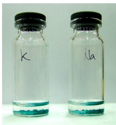
Fig. S23. Photographs of CuHTPO crystals in the vials after CuHTPO crystals were treated in the K + and Na + solution under solvothermal conditions for 100 h.
