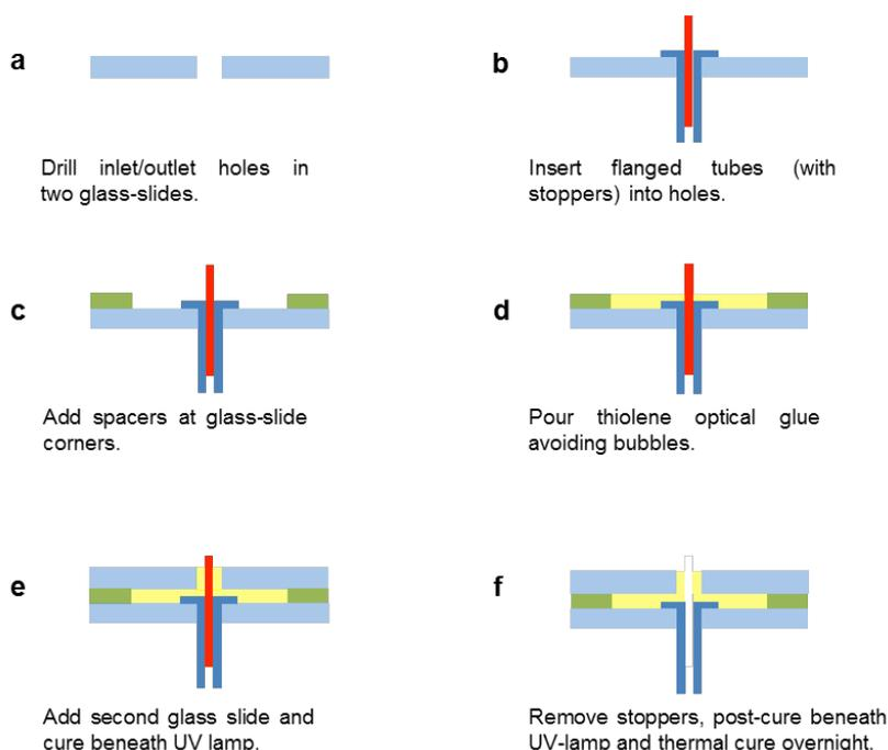
**Fig. S4** Fabrication of the external interface (head of the MR).
