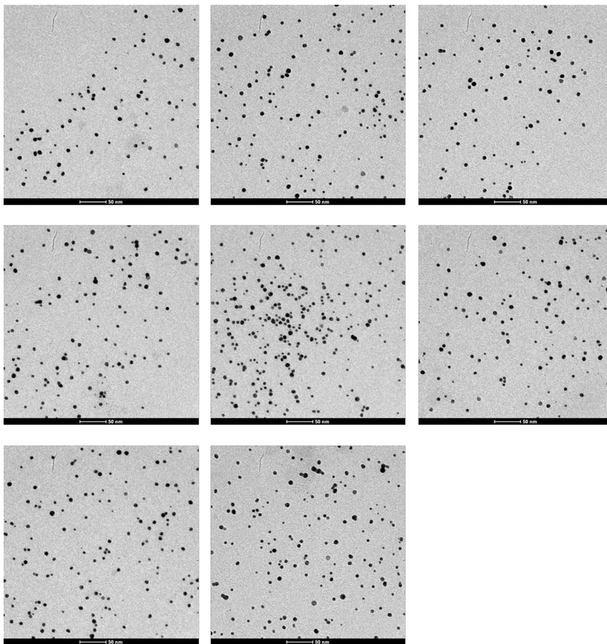
**Fig. S2** TEM images of the silver nanoparticles nucleated in the photoreactor.
