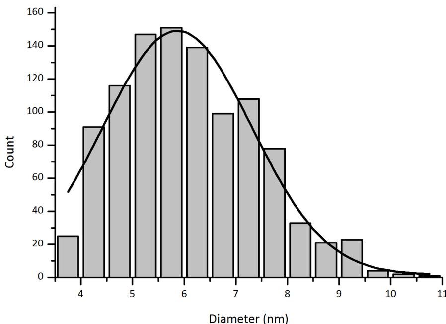
**Fig. S3** Frequency count of the size of the NPs from the images reported in figure S2. The solid line represents the Gaussian fitting, yielding an average size of 5.9 nm.
