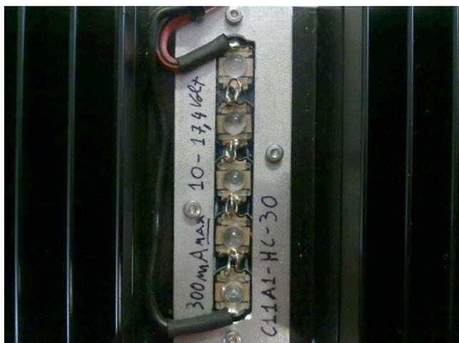
**Fig. S6** Array of 5 LEDs mounted on aluminium heat dissipator.
