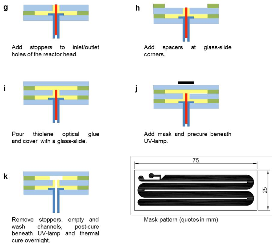
**Fig. S5** Fabrication of the channel network.
