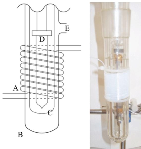
**Fig. S1** Microfluidic photoreactor for the seeding of silver nanoparticles. A Teflon tube (A) was coiled around the external jacket of an immersion photoreactor (B). A high pressure mercury lamp (D), masked by the inner jacket (C) provided the illumination, while being cooled by a water flow entering from (E).
