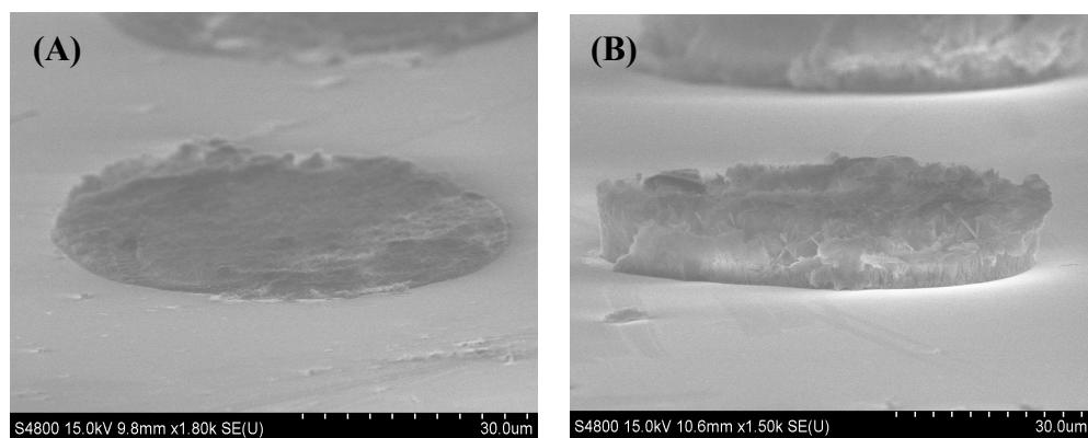
The aqueous solution in the microcapillary contains 1.0 mol/L  $\text{Zn}(\text{NO}_3)_2$  and 0.01 mol/L Hexamethylene tetraamine (HMT), electrodepositing potential: -1.5 V; electrodepositing time: (A) 200s; (B) 400s. With the extending time, the thickness of  $\text{ZnO}$  thin film increases.
