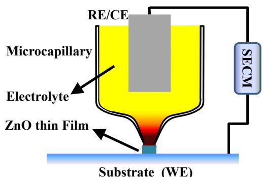
The setup used for electrochemical capacitor experiments is the same as that for ZnO microsynthesis. The difference is that the electrolyte in the microcapillary contains only 0.1 mol/L NaCl. To eliminate the interference from ITO substrate, a newly prepared gold slide was adopted since gold/0.1 mol/L NaCl interface has much smaller double layer charging/discharging background as shown in Fig. 2a of the text.
