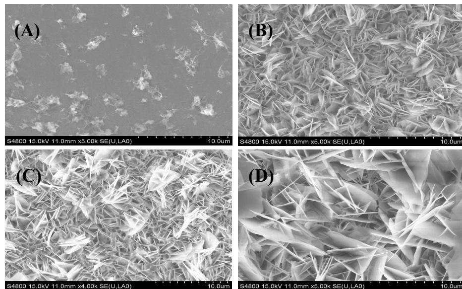
The aqueous solution in the microcapillary contains 1.0 mol/L  $\text{Zn}(\text{NO}_3)_2$  and 0.01 mol/L Hexamethylene tetraamine (HMT), electrodepositing potential: -1.5 V; electrodepositing time: (A) 10s; (B) 100s; (C) 200s; (D) 300s. It's very difficult to get reproducible SEM images before a "monolayer" is formed, i.e., the deposition time is less than 100s in the experimental condition declared in the text (orifice diameter: 50
