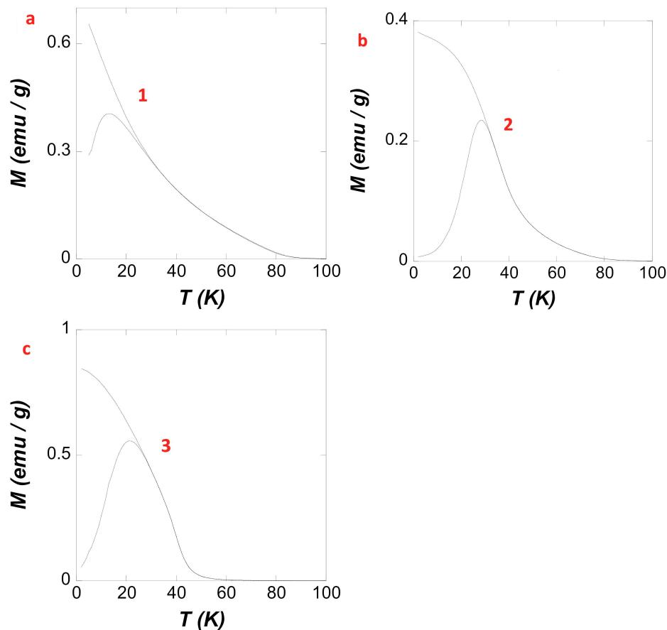
Figure S4. Field and Zero-Field Cooled Magnetization curves for **1**, **2** and **3** measured within an applied field of 30 Oe.
