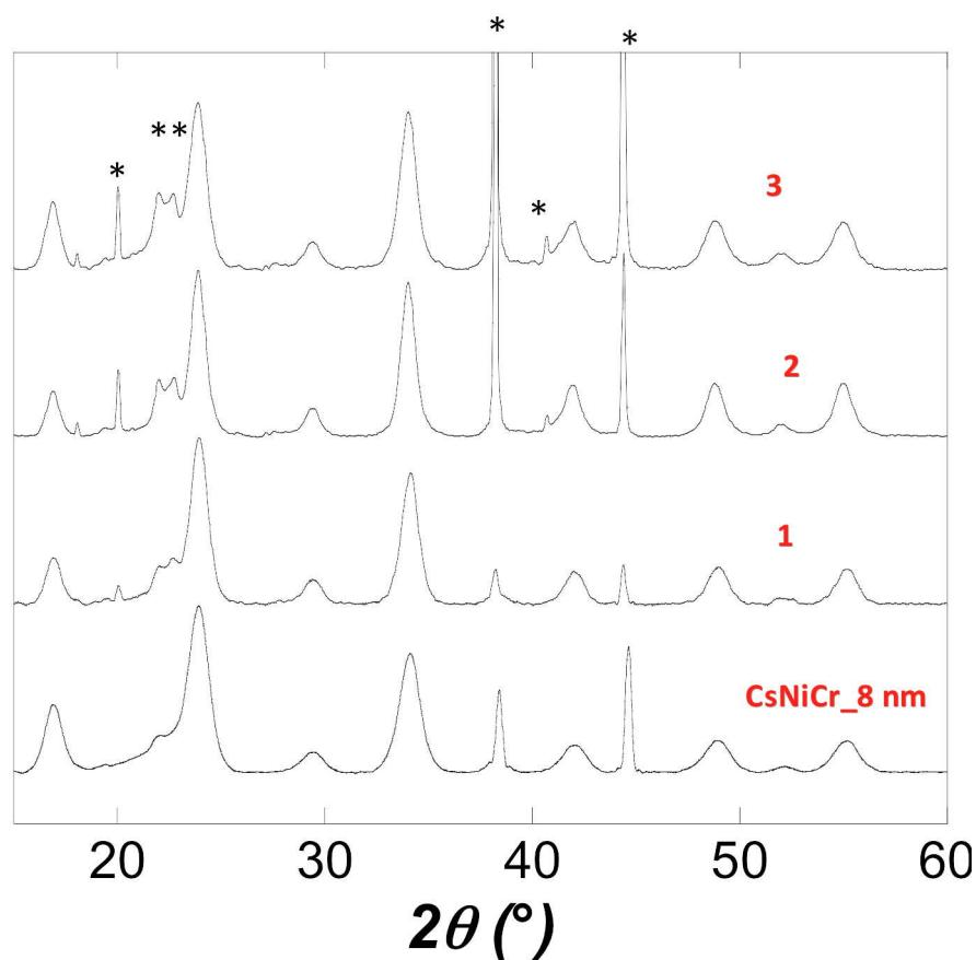
Figure S1. X-ray Powder Diffraction diagrams for the nanoparticles; \*\* indicates the presence of DODABr and \* indicates Al from the sample holder
