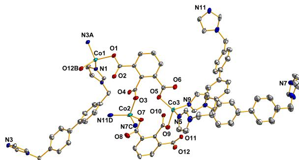
**Fig. S4** The coordination environment of Co(II) atoms in complex **1** with the thermal ellipsoid at the 30% probability level (hydrogen atoms and free water molecules have been omitted for clarity). Symmetry transformations used to generate equivalent atoms:  $A = 1/2 - x, 1/2 - y, z - 1/2$ ,  $B = x, y - 1, z$ ,  $C = x, 2 - y, 1/2 + z$ ,  $D = 1/2 - x, 3/2 - y, 1/2 + z$ .
