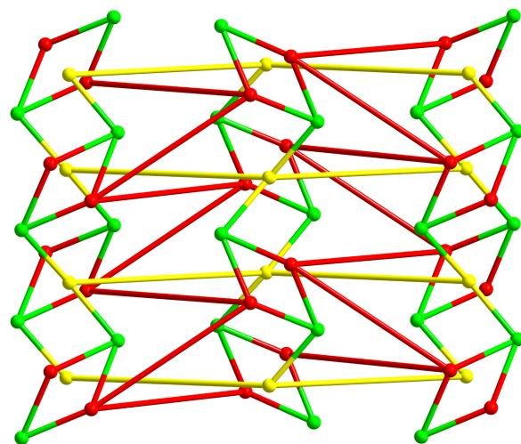
**Fig. S10** Schematic illustrating the 2D (3,4,4)-connected net topological network in 1 (green balls represent the 3-connected btc ligand nodes, yellow balls represent the 4-connected Co1 atoms, red balls represent the 4-connected Co2 and Co3 atoms).
