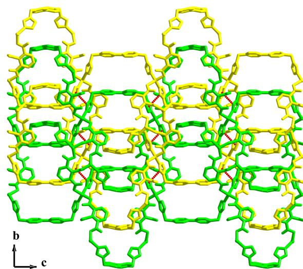
**Fig. S7** The  $\pi$ - $\pi$  interactions (red lines) between imidazole rings in the 2D self-penetrated layers.
