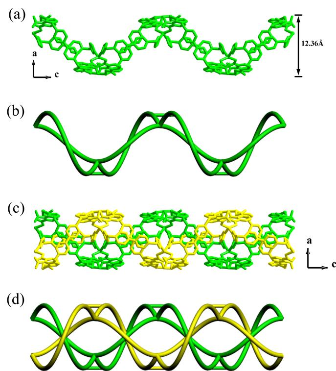
**Fig. S6** A lateral view of the undulating self-penetrating layer (a) and schematic representation (b) of the layer. The interpenetration of pair of the self-penetrating layers (c). Schematic representation of the two-fold interpenetration (d).
