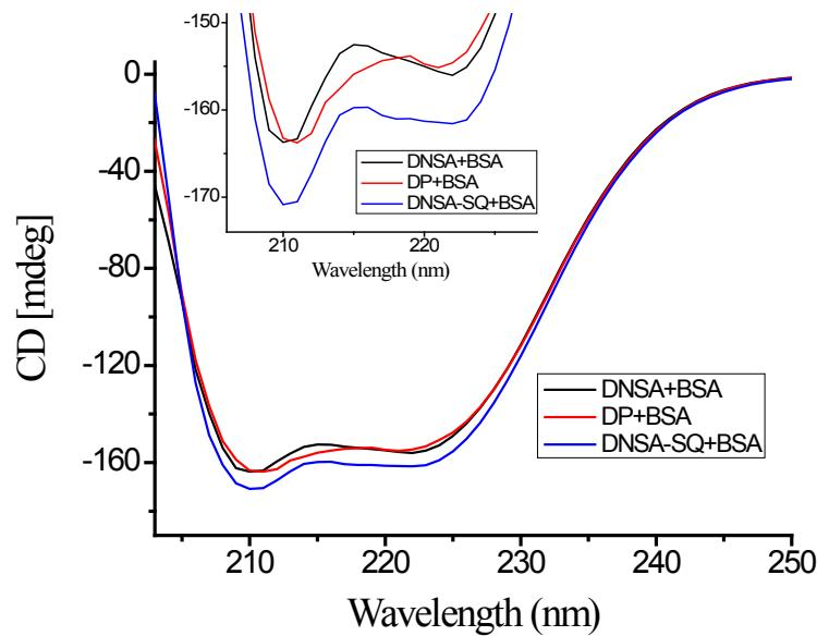
Fig. S9. Circular dichroism of **DNSA-SQ** (2.5  $\mu$ M) in the presence of 1 equiv of BSA.
