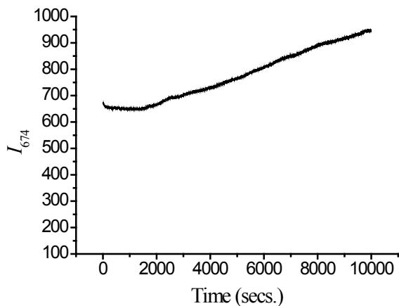
Fig. S17. the fluorescence intensity change of **DNSA-SQ** (5  $\mu$ M) at 674 nm in phosphate buffer solution (10 mM, pH7.2) with 1 equivalent of BSA with increasing reaction time as indicated (excitation wavelength at 600 nm). Within 30 min, the fluorescence intensity of **DNSA-SQ** at 674 nm remains unchanged. Our titration (Figure 2) was recorded within 3 min after BSA was added.
