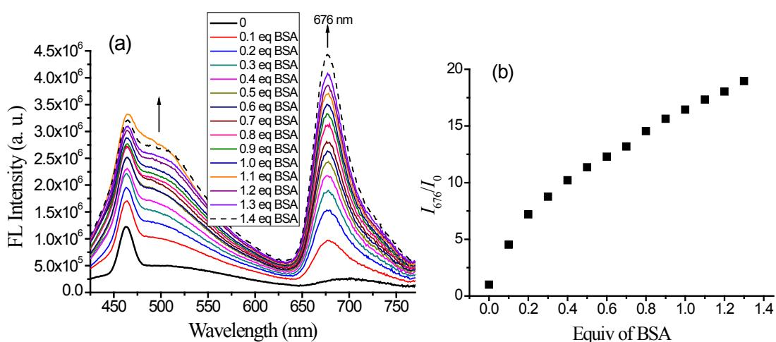
Fig. S8. Fluorescence of **DNSA-SQ** (5  $\mu$ M) in phosphate buffer solution (10 mM, pH 7.2) with different concentration of BSA (a) and relative fluorescence intensity ( $I_{676}/I_0$ ) of **DNSA-SQ** (5  $\mu$ M) at 676 nm (b) in phosphate buffer solution (10 mM, pH 7.2) to different concentration of BSA. (excitation at 400 nm)
