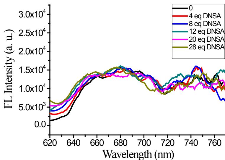
Figure S18. Fluorescence of **DNSA-SQ** (5  $\mu$ M) in phosphate buffer solution (10 mM, pH7.2) with different concentration of DNSA in the absence of BSA (excitation wavelength at 600 nm).
