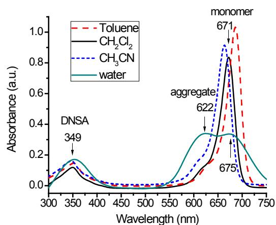
Fig. S4. Absorption of **DNSA-SQ** (5  $\mu\text{M}$ ) in different solvents. The absorption spectrum in water has been multiplied by 4 for clarity.
