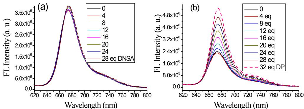
Fig. S11. Fluorescence of **DNSA-SQ** (5  $\mu$ M) in phosphate buffer solution (10 mM, pH 7.2) with different concentration of (a) DNSA and (b) DP in the presence of 3 eq BSA.
