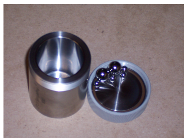
Figure S1. The image of the milling container and balls used in this work.
