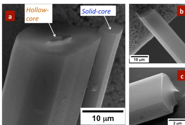
**Figure S4.** (a-c) Morphological inspection revealing the solid-cores of the microwires. These structures are observed along with the more common microtubule structures shown in **Fig. 1** (main text) and **Fig. S3**.
