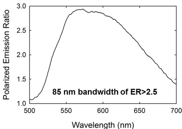
**Figure S8.** Measurement of polarization dependent emission spectrum from the self-assembled microtubules. The polarization ratio is defined to be the ratio of the intensity of linear polarized light in direction of highest linear polarized light intensity to the intensity of linear polarized light 90 degrees from the same direction.
