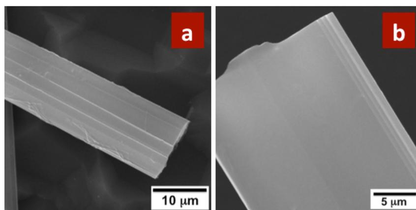
**Figure S5.** (a-b) SEM revealing multi-faceted (> 6) microtubules. These structures are observed along with the ones shown above (**Fig. S3** and **S4**).
