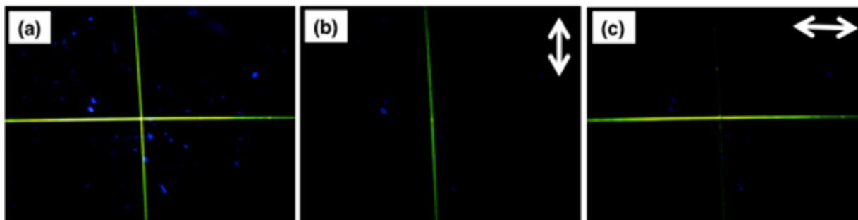
**Figure S7.** Polarized fluorescent emission image from two strategically placed ultra-long microtubules of 1 under excitation from UV-lamp taken from a microscope (a). The strategically placed microtubules emitted linear polarized light. Arrows show the transmission axis of the polarizer placed in front of the camera (b and c).
