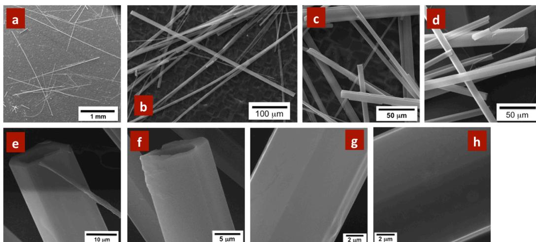
**Figure S3.** More SEM images of the hexagonal faceted microtubules. The most common morphological characteristic observed in the self-assembled structures are hexagonal facet microtubules.
