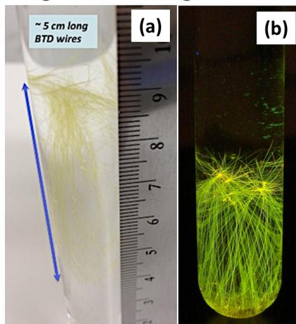
**Figure S2.** Growth of ultra-long microtubules using the phase-transfer method (a) from 1. These ultra-long self-assembled microtubules display strong emission (b) upon excitation under UV-lamp.
