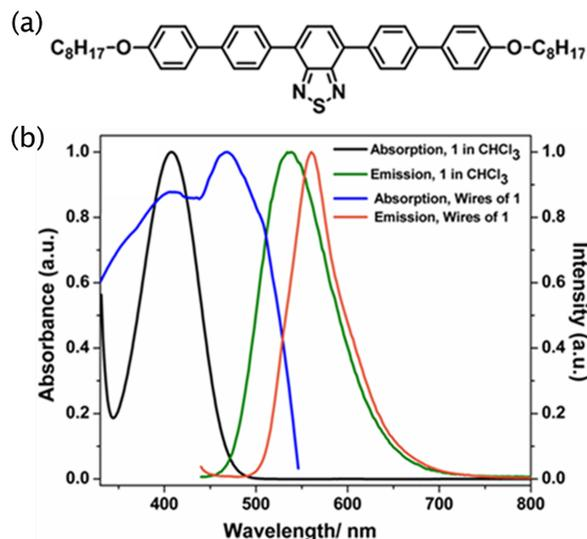
**Figure S1.** (a) Chemical structure of the BTM Absorption and emission characteristics of the BTM molecule in homogeneous solution state (black and green curves) and assembled state (blue and red).
