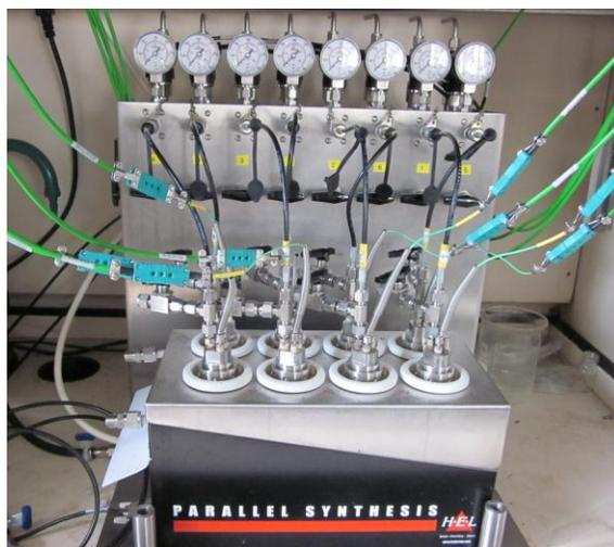
**Figure S1.** Experimental setup of the biocatalytic hydrogenation for carboxylic acids.
