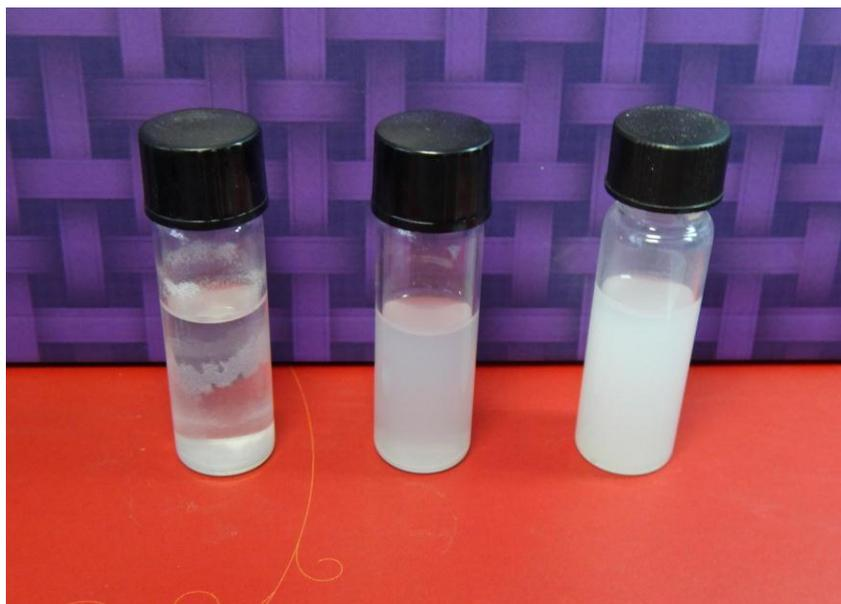
**Fig. S9.** Digital image of SM-*pi*-BNNSs redispersed in cyclohexane, acetone and toluene (from left to right). All the samples were kept for 48 h before photographing. The concentrations of SM-*pi*-BNNSs in acetone and toluene are  $\sim 78$  and  $123 \text{ mg L}^{-1}$  separately as determined by Beer-Lambert plotting at 300 nm [1].
