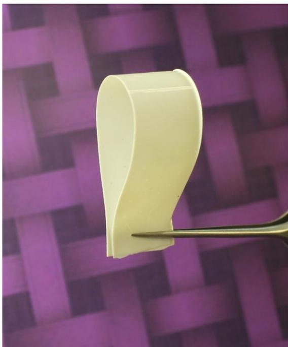
**Fig. S12.** Digital image of an SM-*pi*-BNNSs/PMMA nanocomposite film.
