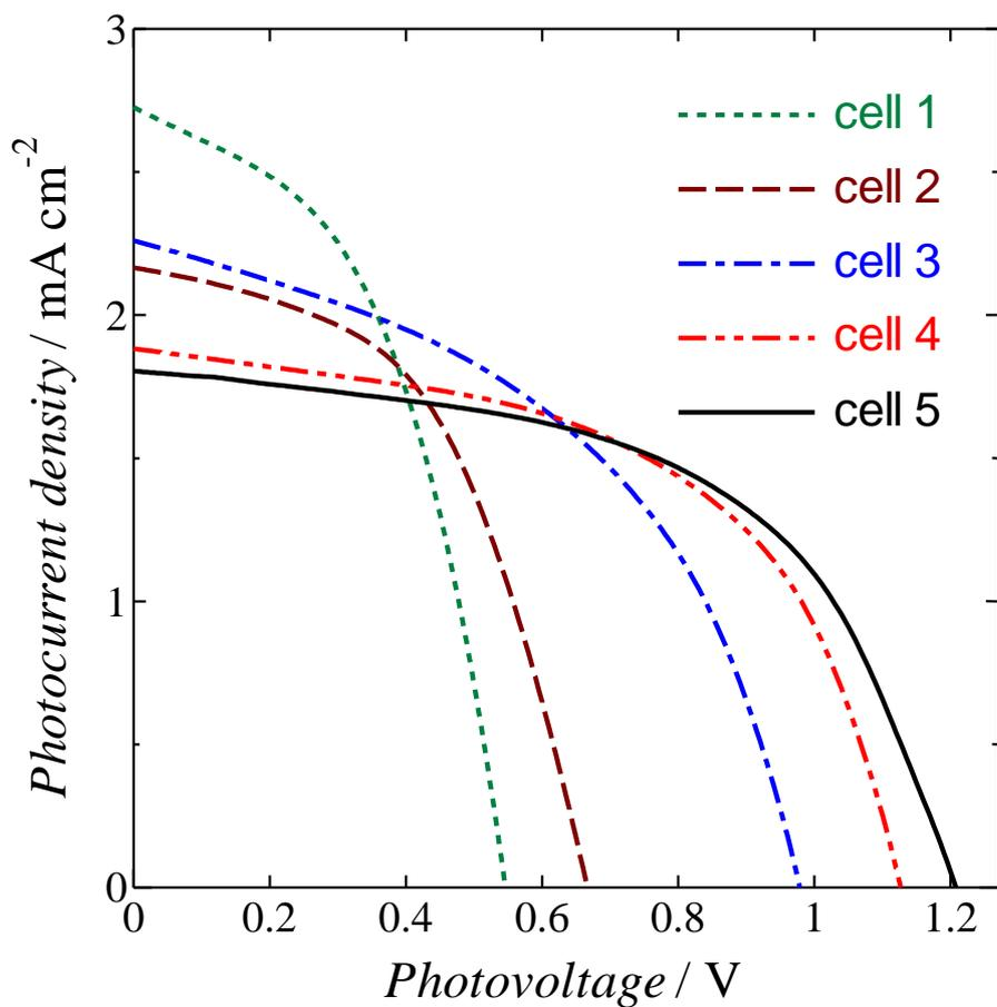
**Figure S2** *I-V* properties of the cells using **SFD-5** as a photosensitizing dye (cell 1-5) under the illumination of the simulated sunlight (AM-1.5G, 100 mW cm<sup>-2</sup>); dotted line represents the result for cell 1, broken line for cell 2, chain line for cell 3, two-dot chain line for cell 4, and solid line for cell 5.
