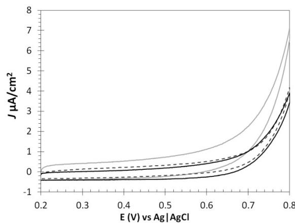
**Fig. S4** Representative cyclic voltammograms of Toray paper electrodes in 0.1 M NaOH solution: Toray paper control in light gray (solid), TBAB modified Nafion coated Toray paper in medium gray (dashed), and magnetic composite in dark gray (solid), stable current response after three cycles at scan rate = 50mV/sec.
