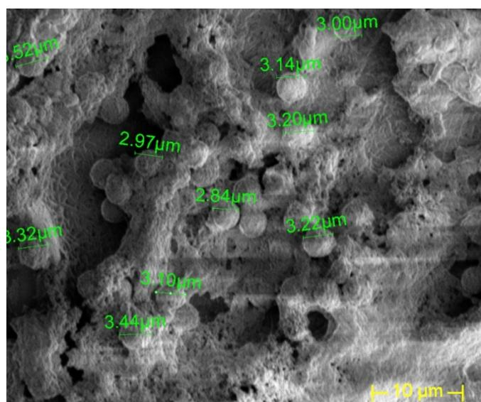
**Fig. S3** SEM of magnetic composite on Toray paper at 6000x magnification and 1 keV; charging evident at this magnification
