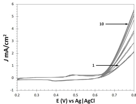
**Fig. S7** Representative cyclic voltammetry of growing-in current response as a function of sweep number with Ni modified Toray paper.
