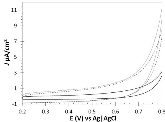
**Fig. S6** Representative cyclic voltammograms of Toray paper electrodes in 0.1 M NaOH solutions / 0.5 M n-butanol: Toray paper control in light gray (solid), TBAB modified Nafion coated Toray paper in medium gray (dashed), and magnetic composite in dark gray (solid), stable current response after three cycles at scan rate = 50mV/sec.
