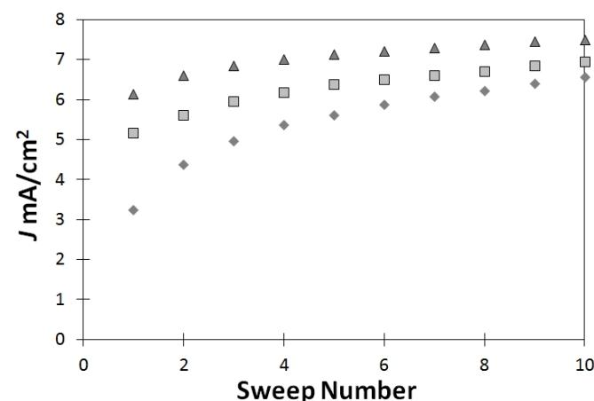
**Fig. S8** Average current response as a function of sweep number in 0.1 M NaOH solution for  $\text{Ni}^{2+}$  deposited Toray paper (diamonds), TBAB modified Nafion coated Ni deposited Toray paper electrodes (squares), and magnetic composite coated Ni deposited Toray paper electrodes (triangles)
