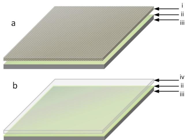
**Figure S1.** Composite electrode schemes, (a.) Magnetic composite, i magnetic microparticles in tetrabutylammonium bromide (TBAB) modified Nafion® film ( $\sim 16\mu\text{m}$ ), ii electrodeposited  $\text{Ni}^{2+}$ , and iii Toray paper; (b.) iv Control TBAB modified Nafion composite, ii electrodeposited  $\text{Ni}^{2+}$ , iii Toray paper.
