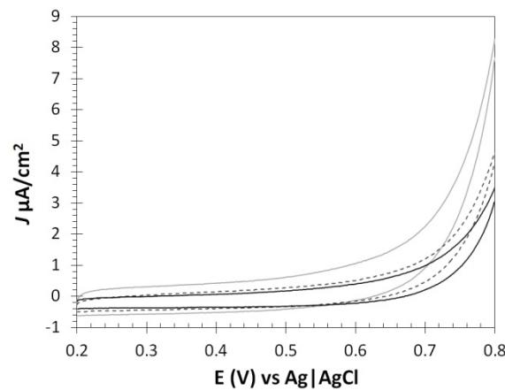
**Fig. S5** Representative cyclic voltammograms of Toray paper electrodes in 0.1 M NaOH / 1 M methanol solution: Toray paper control in light gray (solid), TBAB modified Nafion coated Toray paper in medium gray (dashed), and magnetic composite in dark gray (solid), stable current response after three cycles at scan rate = 50mV/sec.
