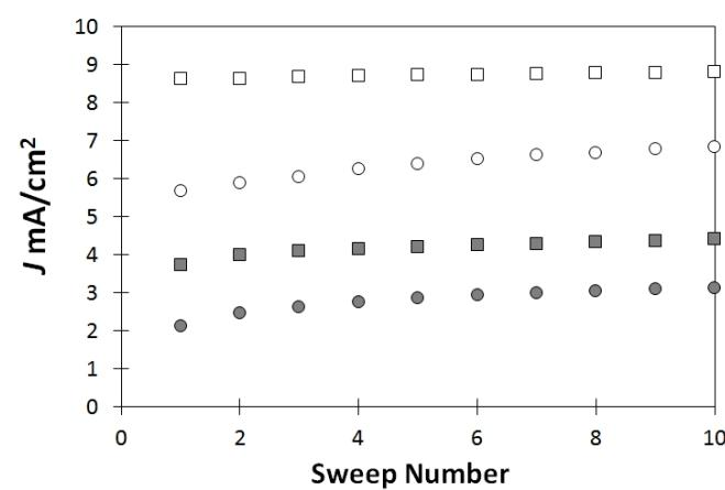
**Fig. S9** Average current response as a function of sweep number in 0.1 M NaOH / 1 M methanol solution for: TBAB modified Nafion coated Ni catalyst electrodes at 0.8 V (gray circle), TBAB Nafion composite electrodes at 0.65 V (white circle), magnetic Nafion composite electrodes at 0.8 V (gray square), and magnetic Nafion composite electrodes at 0.7 V (white square)
