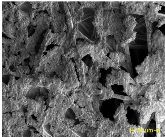
**Fig. S2.** SEM of magnetic composite on Toray paper at 1000x magnification, 1 keV
