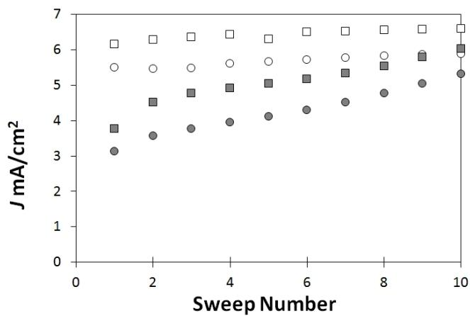
**Fig. S10** Average current response as a function of sweep number in 0.1 M NaOH / 0.5 M n-butanol solution for: TBAB Nafion composite electrodes at 0.8 V (gray circle), TBAB Nafion composite electrodes at 0.65 V (white circle), magnetic Nafion composite electrodes at 0.8 V (gray square), and magnetic Nafion composite electrodes at 0.7 V (white square)
