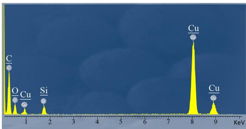
**Figure S7.** Electronic dispersive X-ray spectroscopy (EDS) analysis of as-synthesized HCP@SiO<sub>2</sub>
