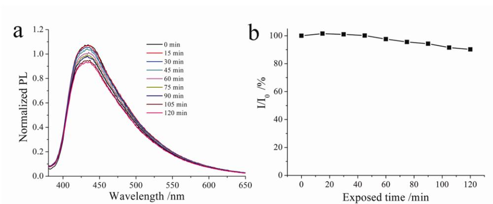
**Figure S13.** The photobleaching curves of HCP@SiO<sub>2</sub> in water under UV lamp with different time.
