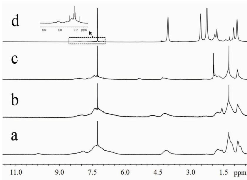
**Figure S1.** <sup>1</sup>H NMR spectra of: (a) HCP-CHO, (b) HCP-OH, (c) HCP-Br, (d) HCP-*star*-PDMAEMA. (400 MHz, in CDCl<sub>3</sub>, 298 K, the solvent is chloroform)
