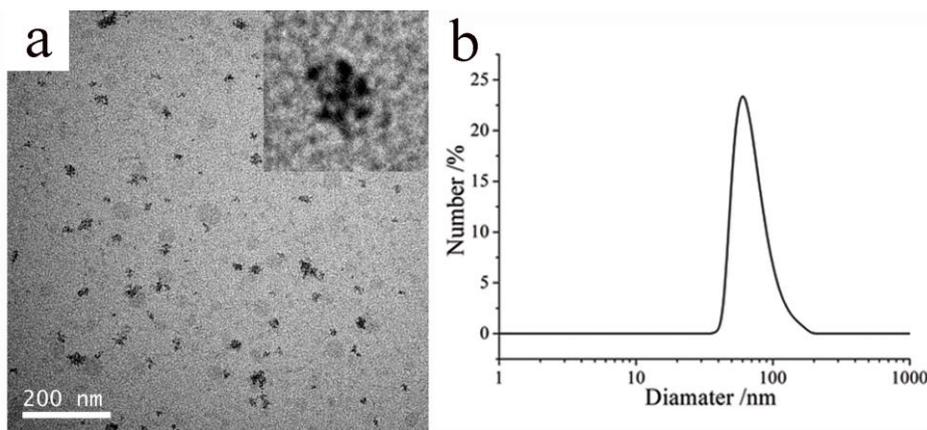
**Figure S10.** TEM photograph (a) and typical number-weighted DLS plot (b) of HCP@SiO<sub>2</sub> aggregates at  $1 \text{ mg mL}^{-1}$  concentration solution in the aqueous medium; the scale bar represents 200 nm for a.
