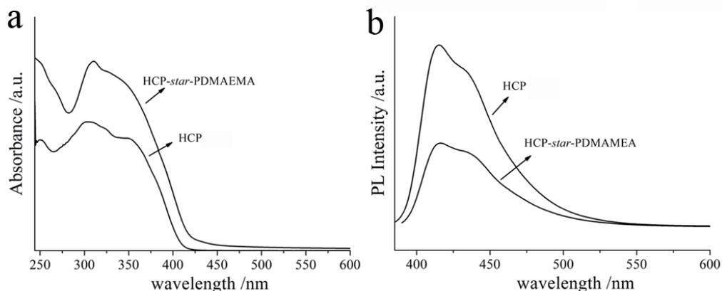
**Figure S8.** The UV-Vis spectra (a) and PL spectra (b) at  $1 \text{ mg mL}^{-1}$  concentration of HCP and HCP-*star*-PDMAEMA in THF solution
