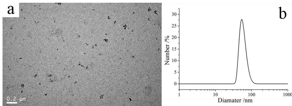
**Figure S14.** (a) TEM photograph and (b) typical number-weighted DLS plot of HCP@SiO<sub>2</sub>-NH<sub>2</sub> aggregates at 1 mg mL<sup>-1</sup> concentration solution in the aqueous medium.
