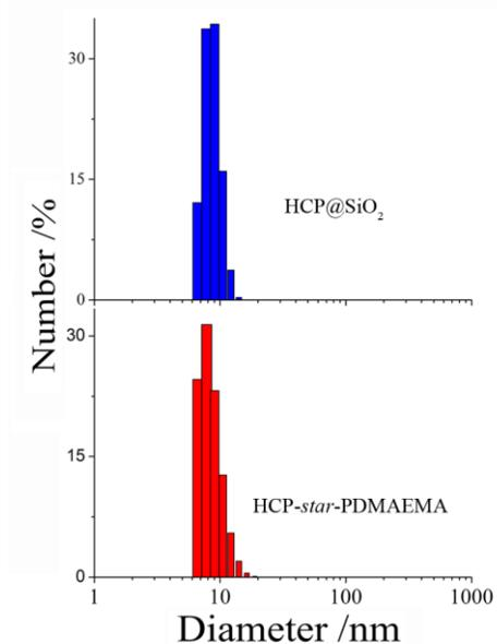
**Figure S6.** Number-averaged size distribution of HCP-*star*-PDMAEMA and as-synthesized HCP@SiO<sub>2</sub> at 0.02 mg mL<sup>-1</sup> concentration solution in THF
