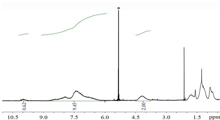
**Figure S3.**  $^1\text{H}$  NMR spectrum of hyperbranched conjugated polymer. (400 MHz, in  $\text{CD}_2\text{Cl}_2$ , 298 K, the solvent peaks are marked with asterisks.)
