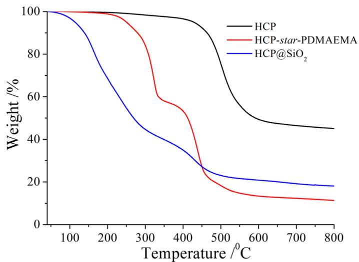
**Figure S5.** The TGA curves of HCP HCP-*star*-PDMAEMA and HCP@SiO<sub>2</sub>.
