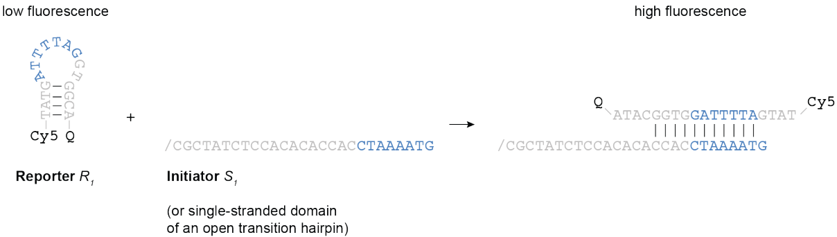
Figure S1. The molecular beacon R_1 is used to report State 1. It is a stem-loop structure labeled at opposite ends with a fluorophore and a quencher (Q). The loop and part of the neck of the R_1 are complementary to the single-stranded sequence that is displayed at the end of the growing polymer when the state machine is in State 1. An increase in fluorescence is seen when the reporter hybridizes to its target sequence because the separation between fluorophore and quencher increases. When the state changes, the molecular beacon is released and the fluorescence signal is quenched as the stem-loop structure refolds. The reporter R_4 is designed to report State 4 in a similar way.
