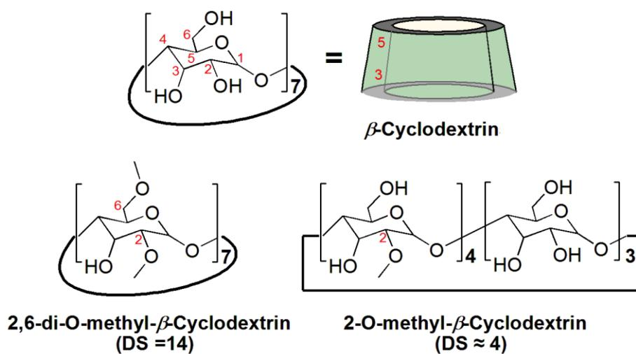
**Figure S1** Chemical structures of  $\beta$ -CD, 2-O-methyl- $\beta$ -CD and 2,6-di-O-methyl- $\beta$ -CD (DS stands for the degree of substitution).
