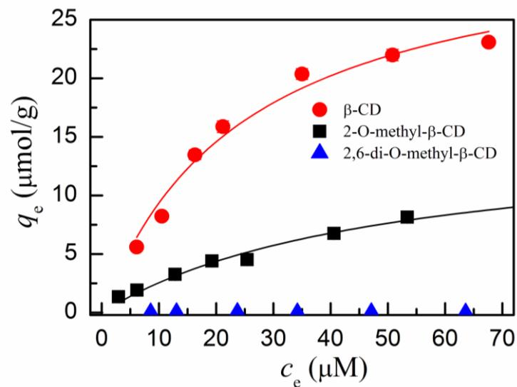
**Figure S2.** Adsorption of  $\beta$ -CD and its derivatives onto  $\text{TiO}_2$  at  $25^\circ\text{C}$ , the lines represent the fit of experimental data to Langmuir isotherm equation.
