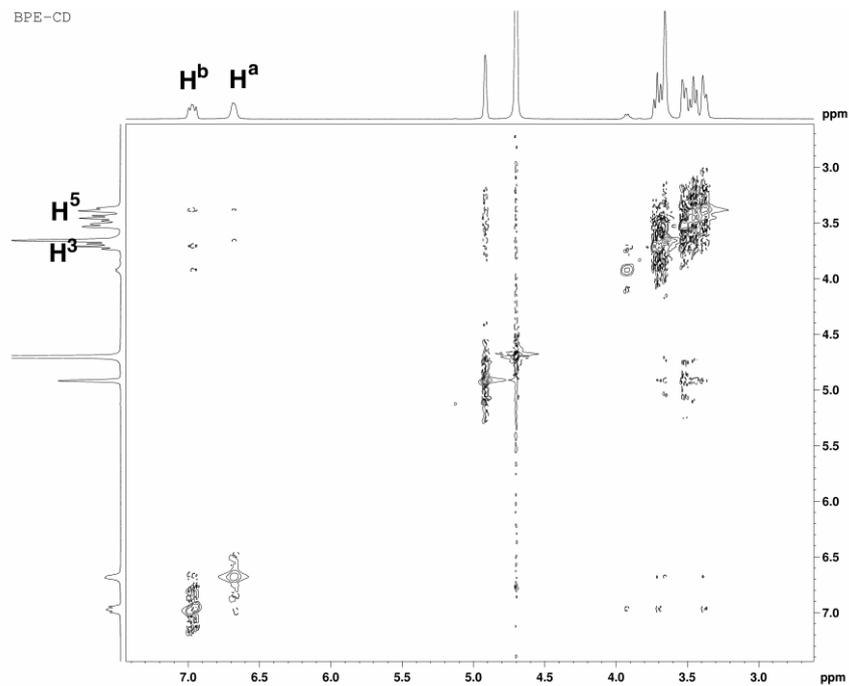
**Figure S3.**  $^1\text{H}$  ROESY spectrum of the  $\beta$ -CD/BPE complex saturated in  $\text{D}_2\text{O}$  at  $25^\circ\text{C}$ .
