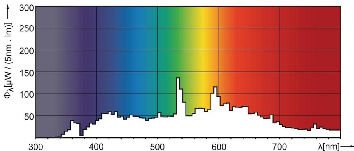
**Figure S5.** The emission spectrum of the Philips Master Color lamp (CDM-T 150W/942)
