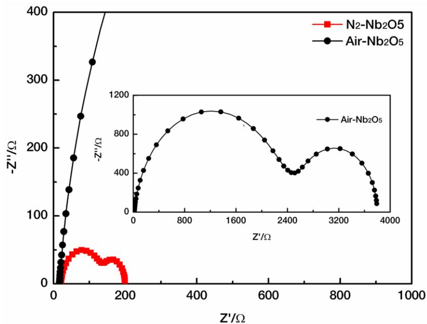
Fig. S1 Electrochemical impedance spectroscopy Nyquist plots of the symmetrical cells using Nb<sub>2</sub>O<sub>5</sub> electrode fabricated in N<sub>2</sub> (■) or air (●) atmosphere, inset is the full scaled Nyquist plot of the Air-Nb<sub>2</sub>O<sub>5</sub>.
