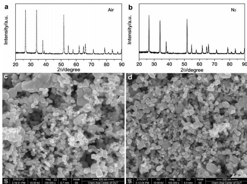
Fig. S2 XRD patterns of the SnO<sub>2</sub> sintered in (a) air and (b) N<sub>2</sub>; SEM image of the SnO<sub>2</sub> sintered in (c) air and (d) N<sub>2</sub>.
