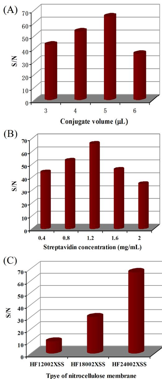
Fig. S2 (A) Effect of the volume of the AuNPs-DNA probe 1 conjugate on the S/N ratio of the strip. (B) Effect of streptavidin concentration (immobilized on the test zone) on the S/N ratio of the strip. (C) Effect of nitrocellulose membrane type on the S/N ratio of the strip.  $\text{Pb}^{2+}$  concentration: 10 nM; volume of the sample solution: 80  $\mu\text{L}$ . All experiments were performed at room temperature.
