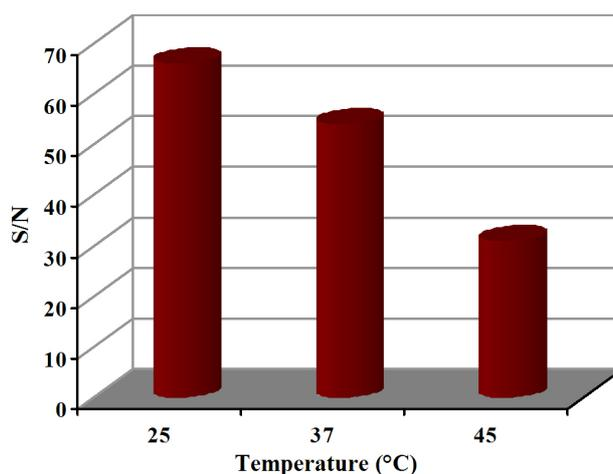
Fig. S1 Effect of the reaction temperature of the catalytic DNA circuit on the S/N ratio of the strip.  $\text{Pb}^{2+}$  concentration: 10 nM; reaction time: 90 min.
