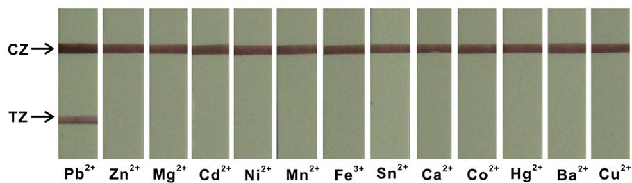
Fig. S3 Selectivity of the strip for  $\text{Pb}^{2+}$  over other competing metal ions. The concentration was 10 nM for  $\text{Pb}^{2+}$  and 500 nM for other metal ions. The incubation time for all metal ions was 90 min.
