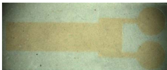
Fig.S-1 A typical photograph of branch electrode.
