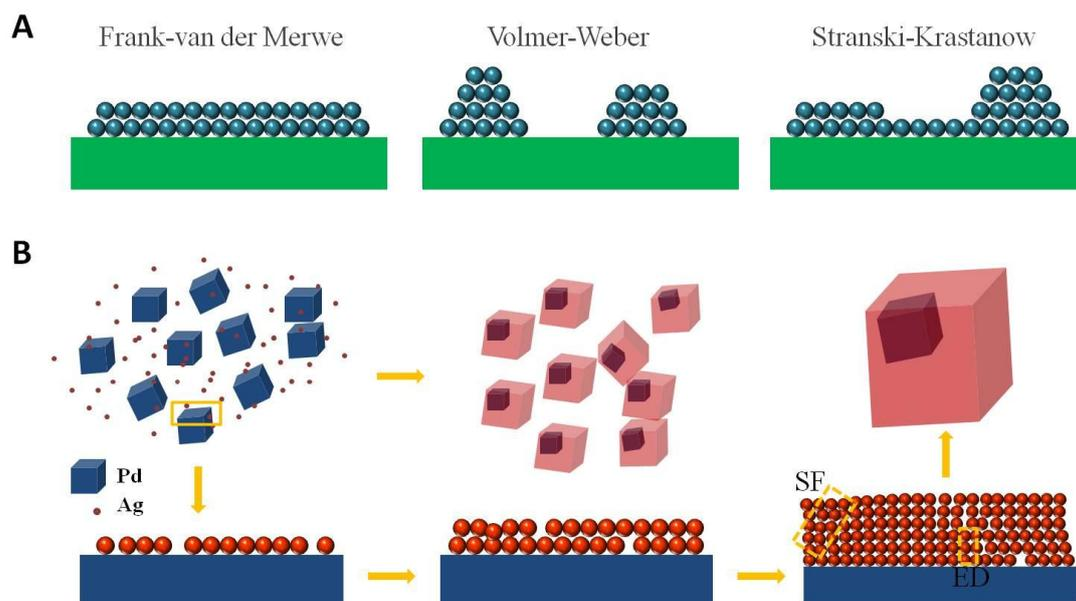
Figure S4. Illustration of the growth mechanism. (A) Three classic growth modes of the films. (B) Growth mechanism of Pd@Ag core-shell NCs.
