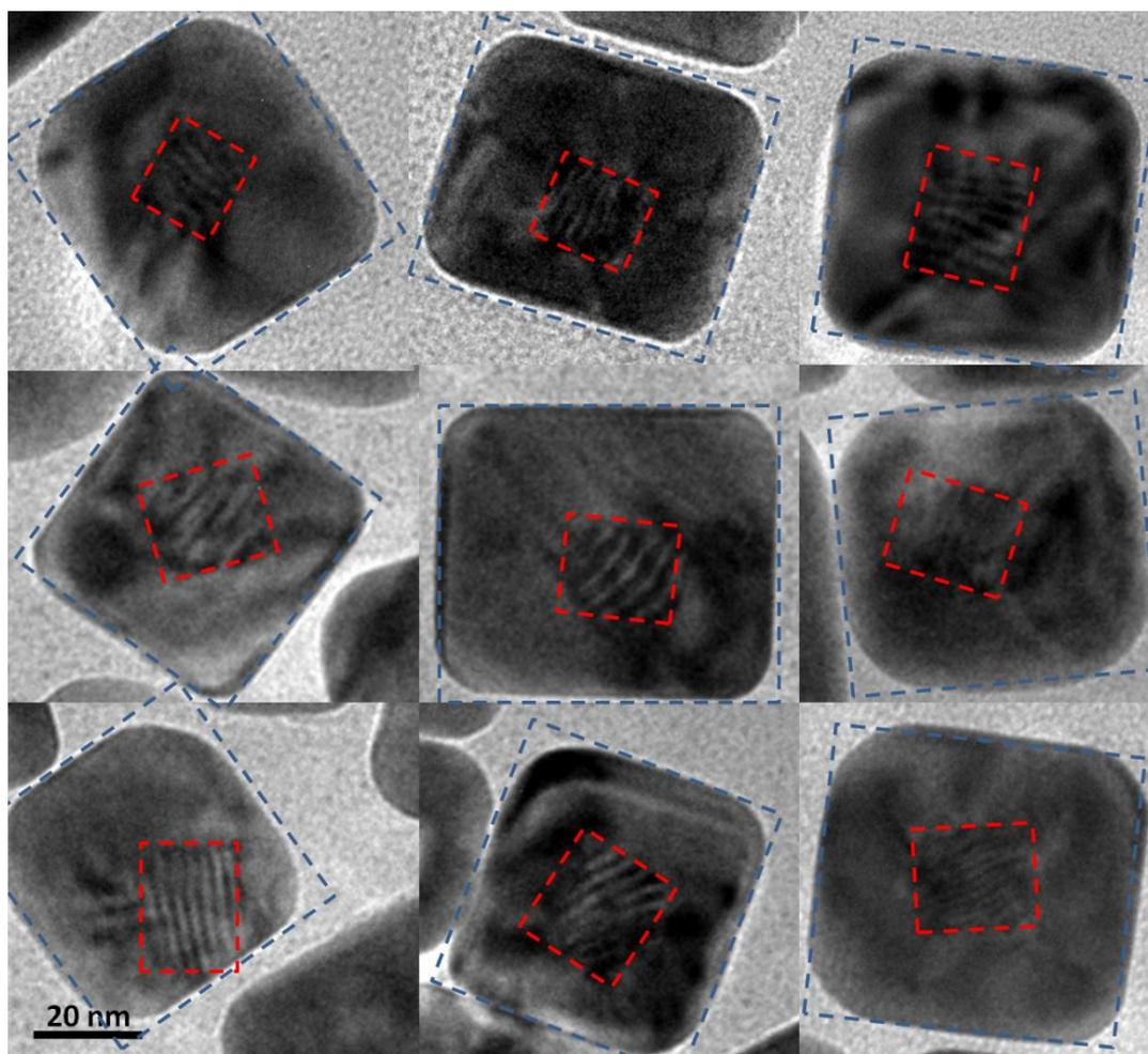
Figure S2. TEM images of individual 50 nm Pd@Ag core-shell NCs. Areas enclosed by blue dotted squares are the position of shells, while areas enclosed by red dotted squares are the position of cores.
