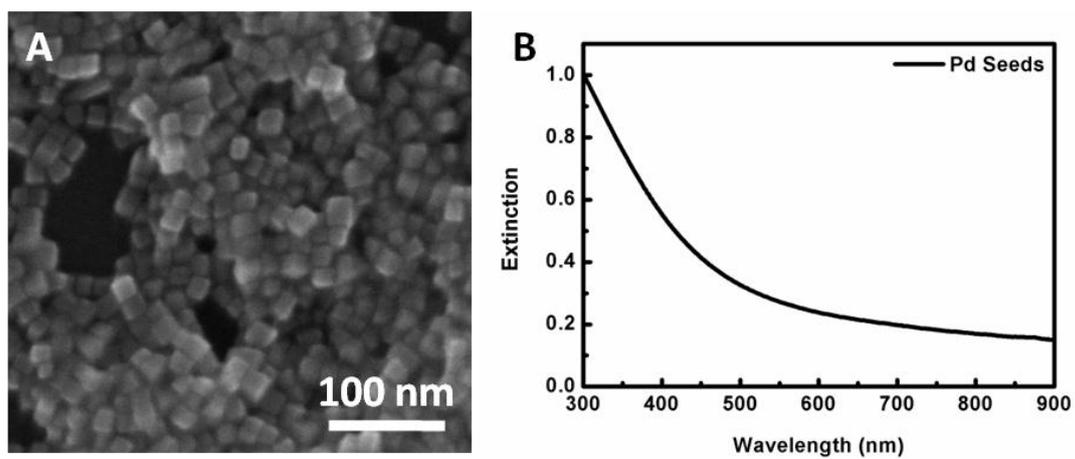
Figure S1. (A) SEM and (B) UV-vis spectrum of Pd seeds.
