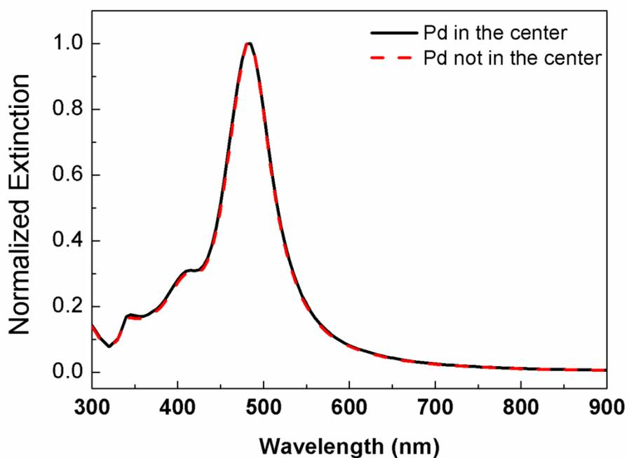
Figure S7. Calculated extinction spectra of 46 nm Pd@Ag nanocrystals with Pd in the center (black solid curve) and in the corner (red dashed curve), respectively. The two curves almost overlap with each other, indicating that the asymmetric arrangement of the core-shell does not significantly change the optical characteristics of the core-shell NCs.
