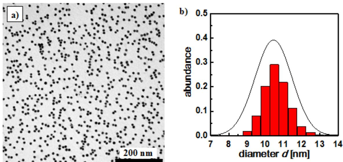
A TEM image of AuNSs is shown in a). For TEM a FEI Technai12 microscope operated at 80 kV was used. For the histogram in b) ImageJ was used and at least 1000 particles were counted. The average diameter of the AuNSs is  $10.4 \pm 0.5$  nm. The line in b) represents a Gaussian fit.
