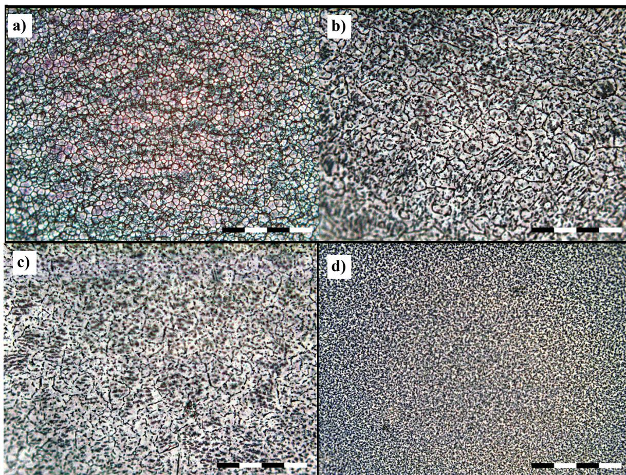
**Figure S3.** Optical microscopy images of the patterned films prepared of blends of 10 nm AuNSs with three different sizes of polymer particles (a) 160 nm, (b) 280 nm, (c) 400 nm and (d) all three sizes of polymer particles. The images were taken from the surface of the dome-like features with an optical microscope and 20x magnification. The volume fraction of the AuNSs is in all cases is  $1.08 \cdot 10^{-4}$ . The scale bars in all images are 100  $\mu\text{m}$ .
