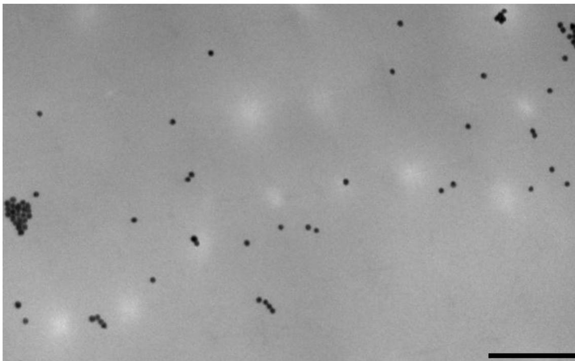
**Figure S5.** TEM cross sectional images of the polymer matrix containing AuNSs. The image shows that the AuNSs are not organised on short (nm) scale. Organization is possible only in longer scales as shown in Figure S3 and S4. Bright dots in the polymer matrix (background) correspond to thinner regions that are remnants of the voids between polymer particles. Scale bar is 200 nm.
