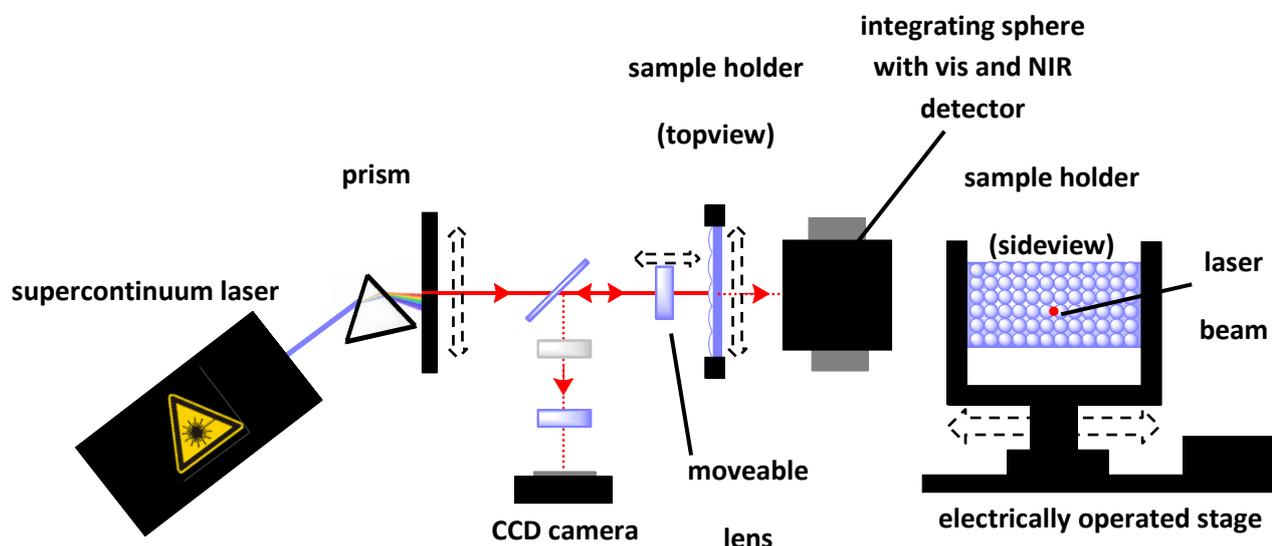
**Figure S1.** Schematic illustration of the technical setup for spatially resolved transmission measurements. The moveable elements are marked by the dashed arrows. The sample holder is placed on a lateral moveable stage, which enables spatially resolved measurements with a  $50 \mu\text{m}$  resolution.
