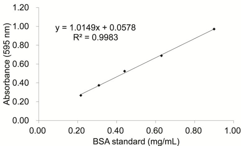
**Figure S3.** The calibration curve of the Bradford assay. The purified BSA standard solution was diluted producing concentrations varying from 0.20 to 1.00 mg/mL, at an interval of 0.20 mg/mL. The UV-vis absorbance at 595 nm was measured after BSA standards were mixed with dye solutions at rt for 10 min.
