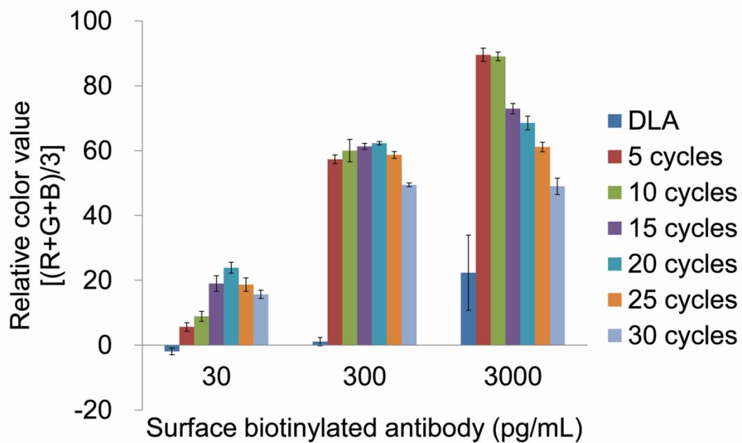
**Figure S12.** Comparison of the DLA and SBPN (5-30 cycles) methods performed on a biotinylated antibody coated surface using normalized data. Normalization was achieved by subtracting the average background signal from the average relative color values of each experiment.
