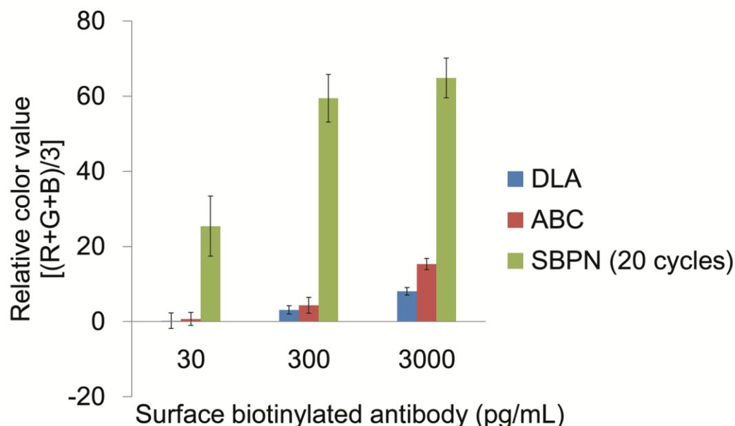
**Figure S14.** Comparison of the ABC, DLA, and SBPN (20 cycles) methods performed on a biotinylated antibody coated surface using normalized data. Normalization was achieved by subtracting the average background signal from the average relative color values of each experiment (average of 9 total data points).
