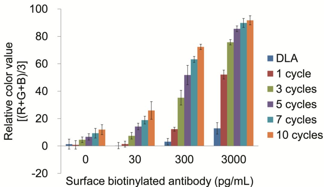
**Figure S5.** Comparison of the DLA and SBPN (1-10 cycles) methods. Various concentrations of biotinylated antibodies are plotted versus the average of relative color values. Error bars indicate  $\pm 1$  standard deviation. The plot was generated from the data shown in Table S3. The relative color values become larger when the number of cycles is increased.
