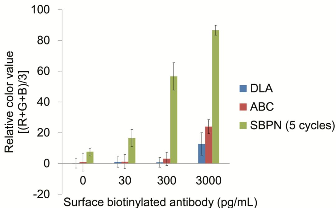
**Figure S16.** Comparison of the ABC, DLA, and SBPN (5 cycles) methods performed on a biotinylated antibody coated surface. Various concentrations of biotinylated antibodies are plotted versus the average of relative color values. Error bars indicate  $\pm 1$  standard deviation. The plot was generated from the data shown in Table S9.
