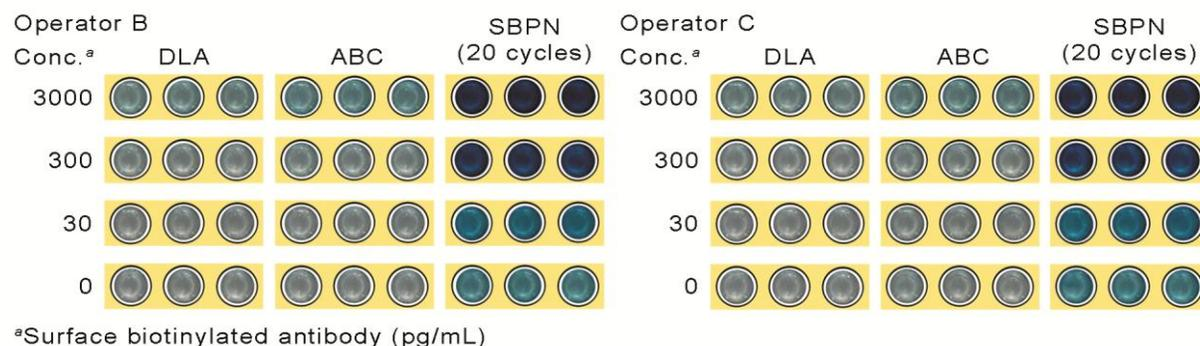
**Figure S13.** Comparison among the ABC, DLA, and SBPN (20 cycles) methods performed on a biotinylated antibody coated surface. These experiments were performed by three different technicians. The SBPN method produces the strongest signal among three methods. A detailed discussion is provided in the manuscript.
